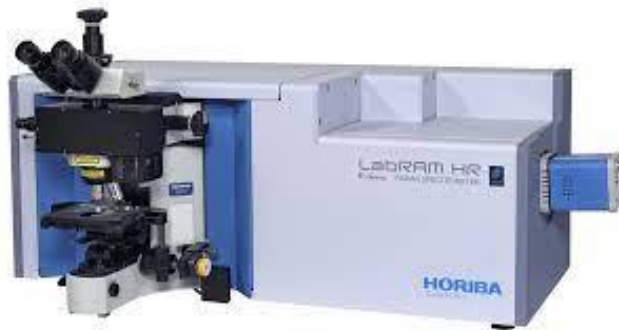
Figure 2.7: LABRAM Horiba Raman Spectroscopy Setup - CIGS UNIMORE
