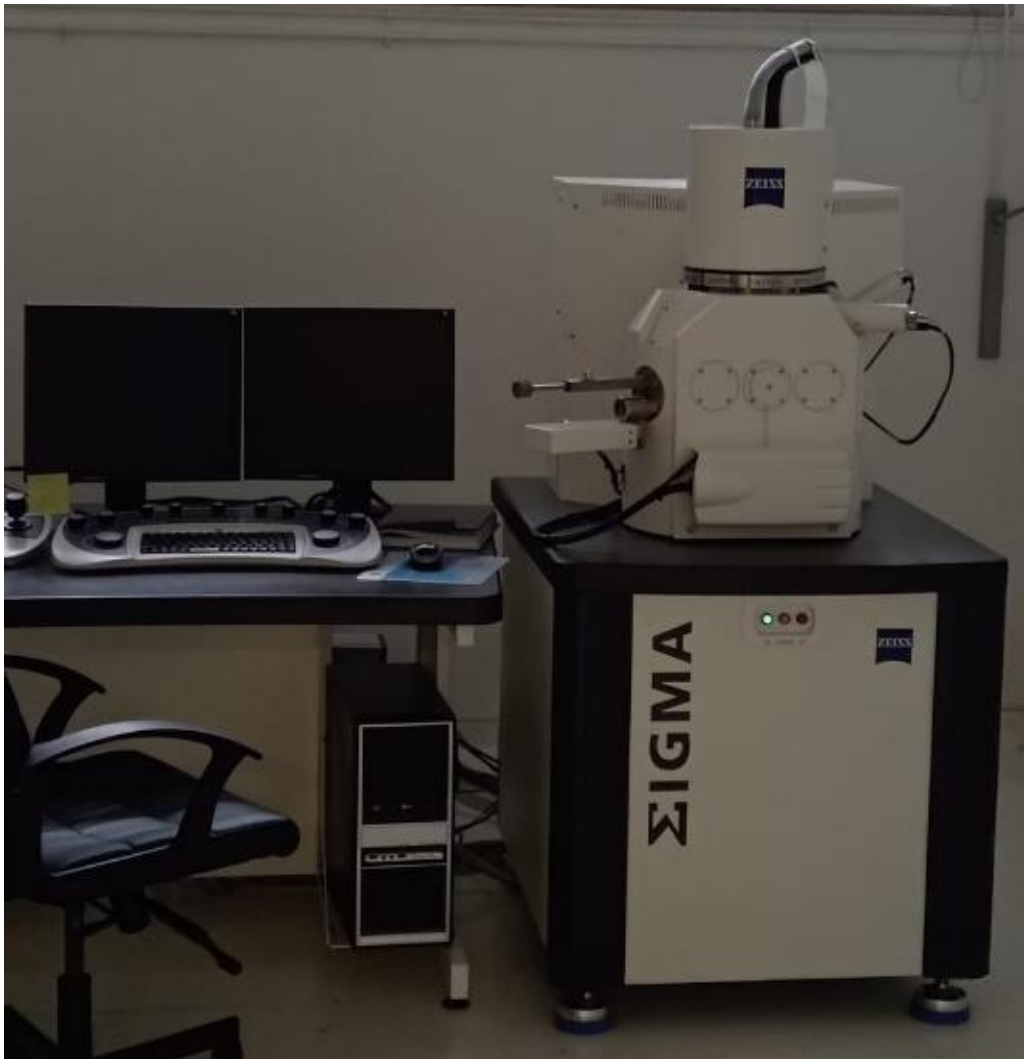
Figure 2.12: ZEISS Electron Beam Lithography Setup -Nanofabrication Facility -Physics Department-UNIMORE
