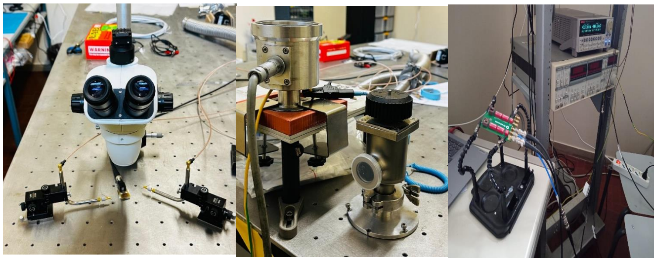
Figure 2.19: Electrical Transport Measurement setup under ambient conditions, vacuum and for the packaged device with Graphenea Card
