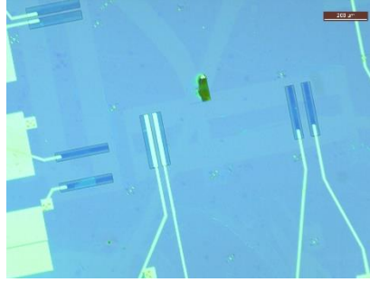
Figure 2.10: Multiple Fabricated Devices on single CVD graphene substrate by Electron Beam Lithography
