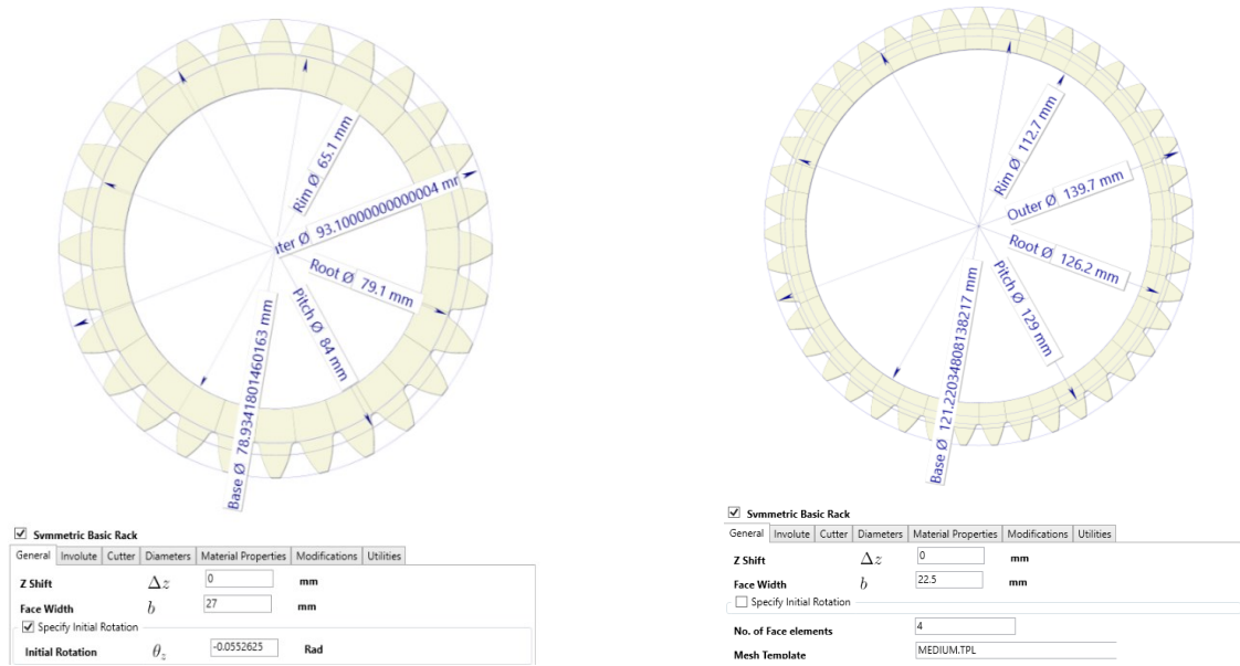
Figure 3 geometrical and material characteristics of the gear pair
