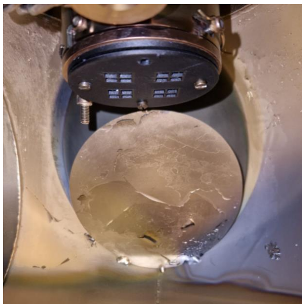
Figure 128 The steps involved in assembling and using the custom-made a) Sample holder of the evaporator b) The base of the mask is coupled to the sample holder c) The glass slides are positioned within the designated slots d) The mask cover is secured e) The sample holder, connected to the mask, is positioned in the evaporation chamber f) At the end of the process, the sample holder is removed from the chamber
