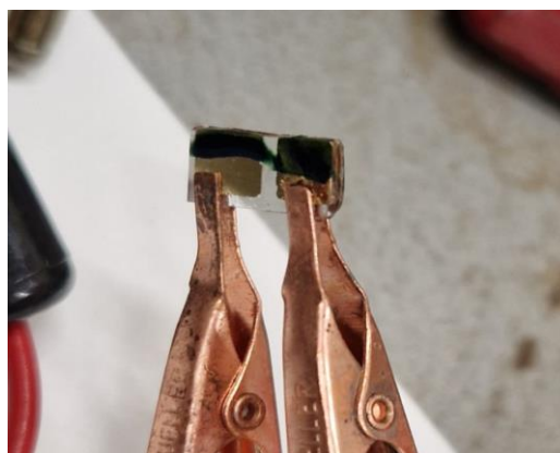
Figure 99 a) two-Au pads substrates for the preparation of Au|PANI samples suitable for transport measurements (electrical characterization in a 4-point configuration) b) sample obtained at the end of the electropolymerization process.
