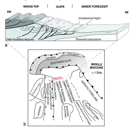
**Figure 2.** (a) Block diagram showing the northern Apennine wedge-foredeep system during the Miocene. Seep carbonates occurred in wedge-top basins, on the slope and in the inner foredeep basin. (b) Simplified paleogeographic sketch of the Apennine domains during the middle Miocene (modified from [26]).
