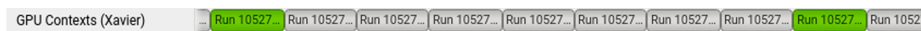
Fig. 12. GPU context switch when more process uses the GPU. Green slots are the path planner process, grey slots are other interference processes.
