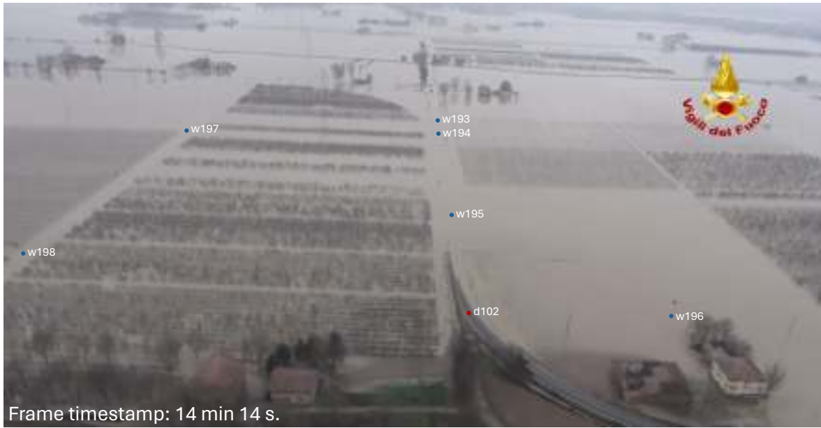
Figure S73. Frame of the aerial videography taken by the “Vigili del Fuoco” Fire Department of Modena. Wet points are highlighted in blue and dry points are highlighted in red. The time reported in the frame is counted from the beginning of the aerial videography occurred on 20 January 2014 at about 11:30 AM.
