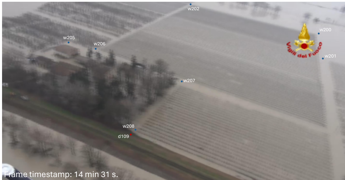
Figure S75. Frame of the aerial videography taken by the “Vigili del Fuoco” Fire Department of Modena. Wet points are highlighted in blue and dry points are highlighted in red. The time reported in the frame is counted from the beginning of the aerial videography occurred on 20 January 2014 at about 11:30 AM.
