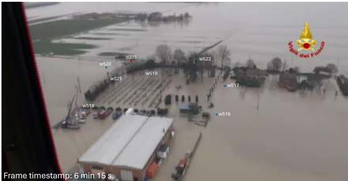
Figure S17. Frame of the aerial videography taken by the “Vigili del Fuoco” Fire Department of Modena. Wet points are highlighted in blue and dry points are highlighted in red. The time reported in the frame is counted from the beginning of the aerial videography occurred on 20 January 2014 at about 11:30 AM.
