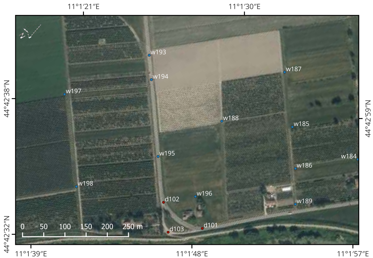
Figure S72. Orthoimage associated to the previous aerial videography frame, where georeferenced wet points are highlighted in blue and georeferenced dry points are highlighted in red.
