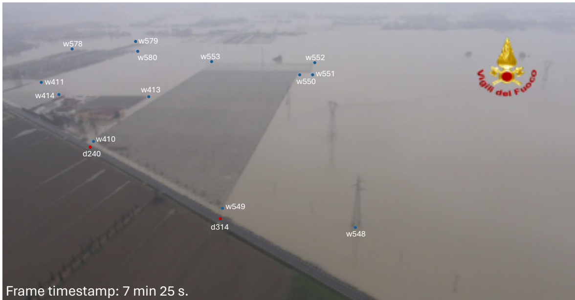
Figure S25. Frame of the aerial videography taken by the “Vigili del Fuoco” Fire Department of Modena. Wet points are highlighted in blue and dry points are highlighted in red. The time reported in the frame is counted from the beginning of the aerial videography occurred on 20 January 2014 at about 11:30 AM.
