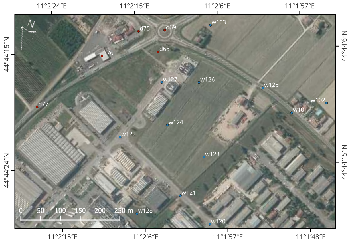
Figure S52. Orthoimage associated to the previous aerial videography frame, where georeferenced wet points are highlighted in blue and georeferenced dry points are highlighted in red.
