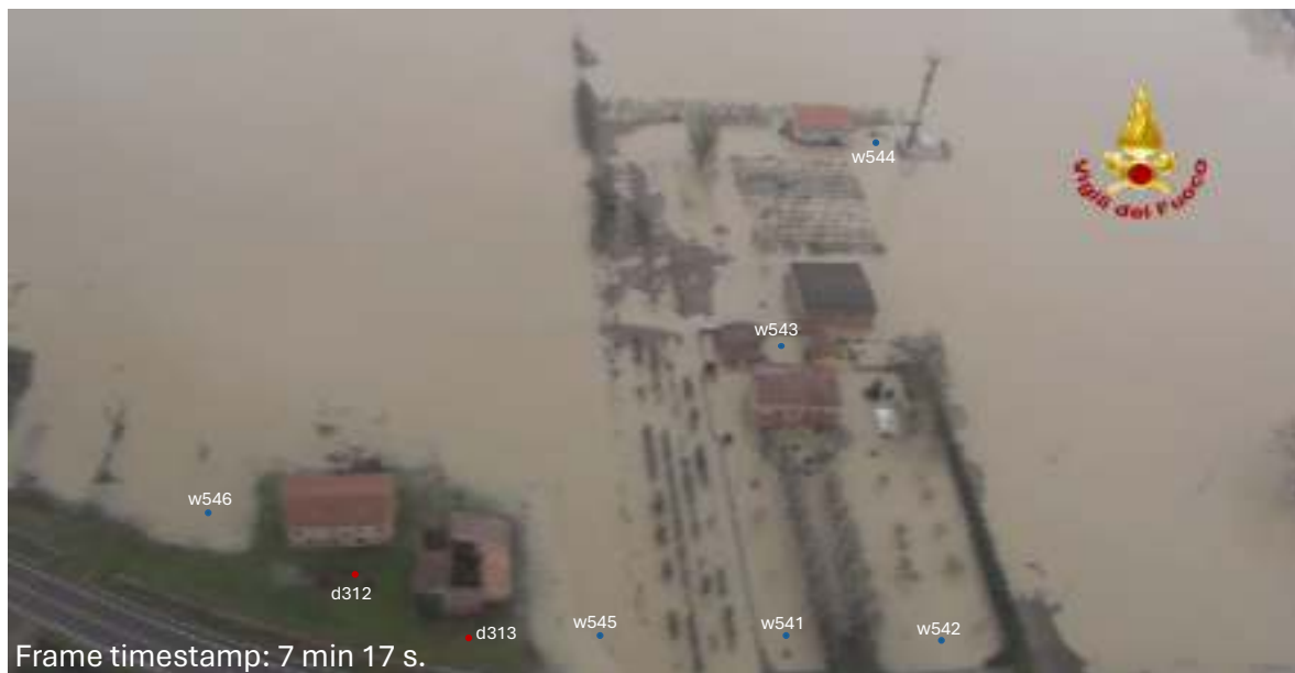
Figure S23. Frame of the aerial videography taken by the “Vigili del Fuoco” Fire Department of Modena. Wet points are highlighted in blue and dry points are highlighted in red. The time reported in the frame is counted from the beginning of the aerial videography occurred on 20 January 2014 at about 11:30 AM.
