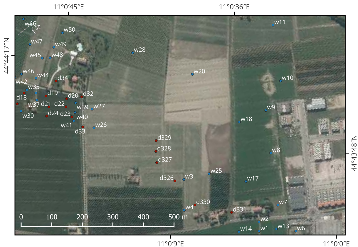
Figure S40. Orthoimage associated to the previous aerial videography frame, where georeferenced wet points are highlighted in blue and georeferenced dry points are highlighted in red.
