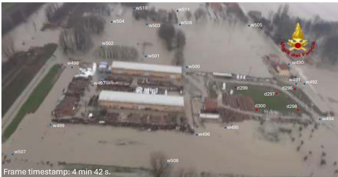
Figure S13. Frame of the aerial videography taken by the “Vigili del Fuoco” Fire Department of Modena. Wet points are highlighted in blue and dry points are highlighted in red. The time reported in the frame is counted from the beginning of the aerial videography occurred on 20 January 2014 at about 11:30 AM.
