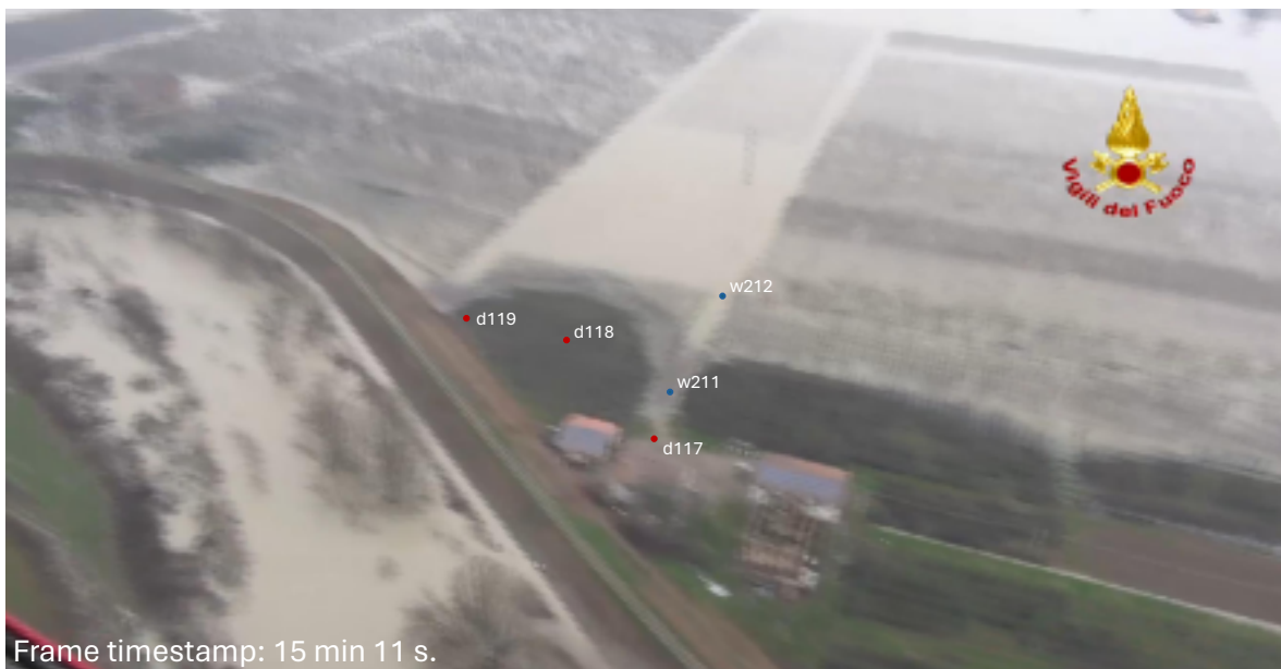
Figure S81. Frame of the aerial videography taken by the “Vigili del Fuoco” Fire Department of Modena. Wet points are highlighted in blue and dry points are highlighted in red. The time reported in the frame is counted from the beginning of the aerial videography occurred on 20 January 2014 at about 11:30 AM.
