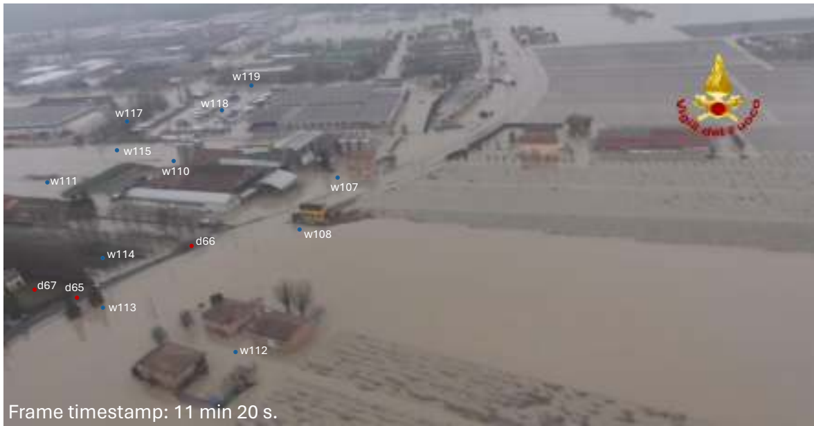
Figure S49. Frame of the aerial videography taken by the “Vigili del Fuoco” Fire Department of Modena. Wet points are highlighted in blue and dry points are highlighted in red. The time reported in the frame is counted from the beginning of the aerial videography occurred on 20 January 2014 at about 11:30 AM.
