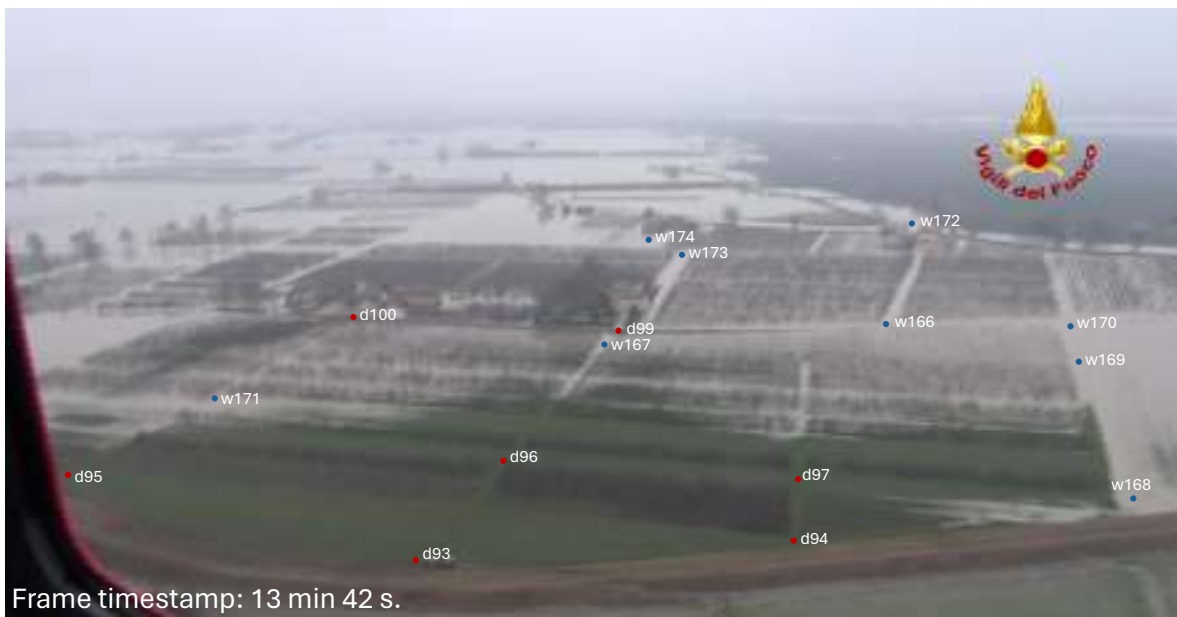
Figure S67. Frame of the aerial videography taken by the “Vigili del Fuoco” Fire Department of Modena. Wet points are highlighted in blue and dry points are highlighted in red. The time reported in the frame is counted from the beginning of the aerial videography occurred on 20 January 2014 at about 11:30 AM.
