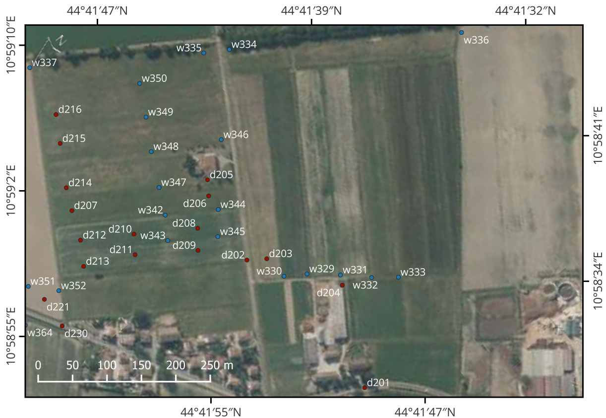
Figure S108. Orthoimage associated to the previous aerial videography frame, where georeferenced wet points are highlighted in blue and georeferenced dry points are highlighted in red.
