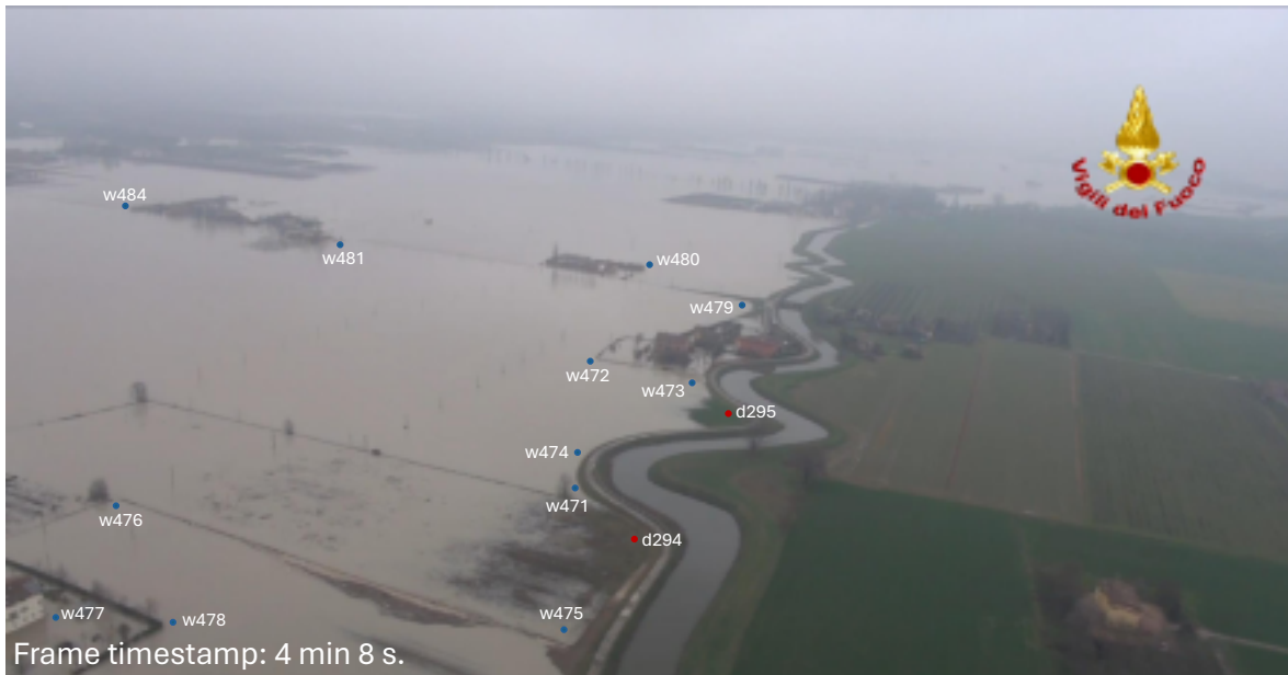
Figure S9. Frame of the aerial videography taken by the “Vigili del Fuoco” Fire Department of Modena. Wet points are highlighted in blue and dry points are highlighted in red. The time reported in the frame is counted from the beginning of the aerial videography occurred on 20 January 2014 at about 11:30 AM.
