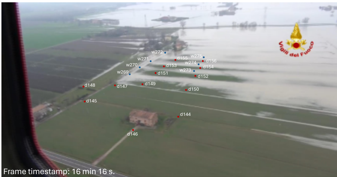
Figure S95. Frame of the aerial videography taken by the “Vigili del Fuoco” Fire Department of Modena. Wet points are highlighted in blue and dry points are highlighted in red. The time reported in the frame is counted from the beginning of the aerial videography occurred on 20 January 2014 at about 11:30 AM.
