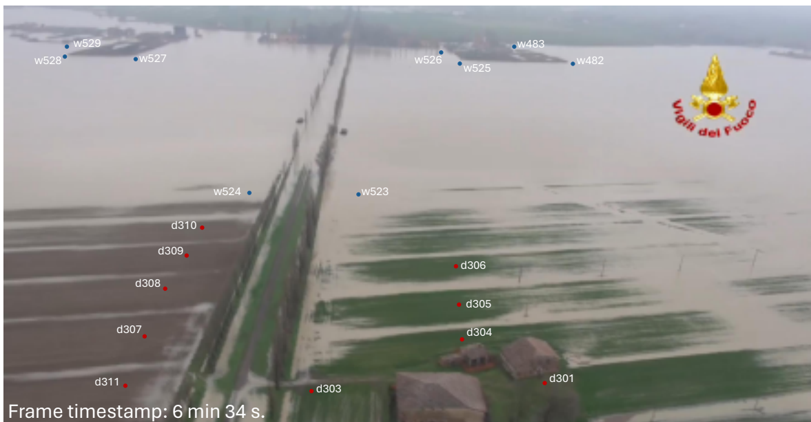
Figure S19. Frame of the aerial videography taken by the “Vigili del Fuoco” Fire Department of Modena. Wet points are highlighted in blue and dry points are highlighted in red. The time reported in the frame is counted from the beginning of the aerial videography occurred on 20 January 2014 at about 11:30 AM.
