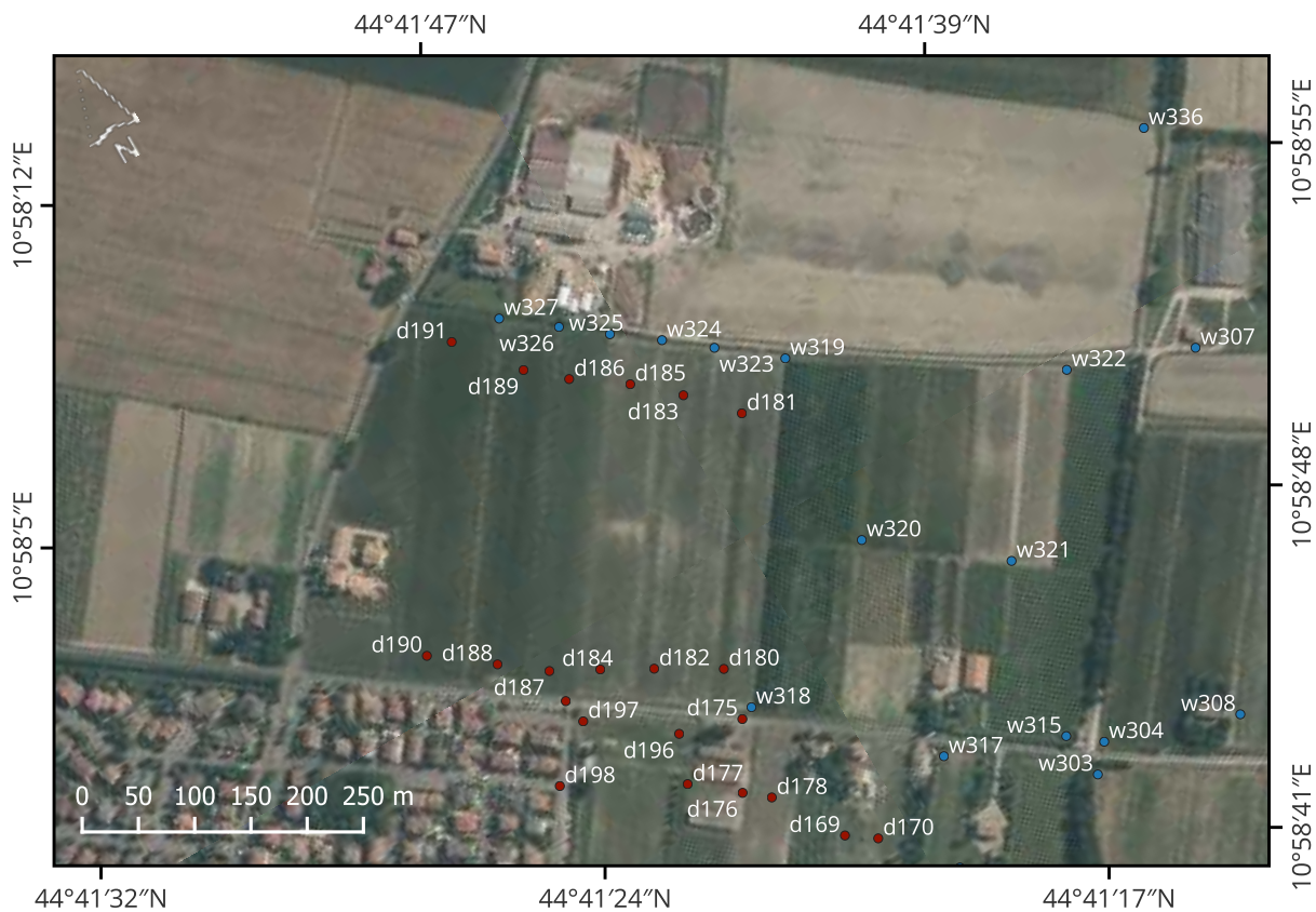
Figure S106. Orthoimage associated to the previous aerial videography frame, where georeferenced wet points are highlighted in blue and georeferenced dry points are highlighted in red.
