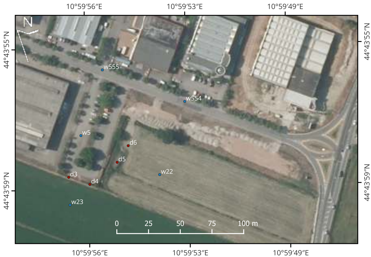
Figure S30. Orthoimage associated to the previous aerial videography frame, where georeferenced wet points are highlighted in blue and georeferenced dry points are highlighted in red.
