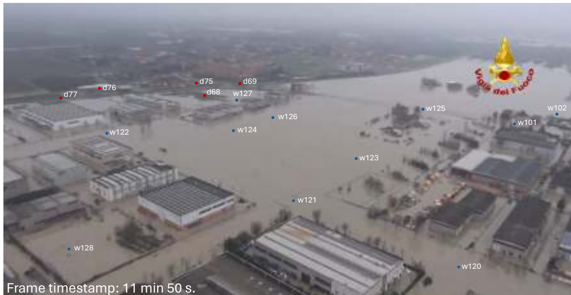
Figure S51. Frame of the aerial videography taken by the “Vigili del Fuoco” Fire Department of Modena. Wet points are highlighted in blue and dry points are highlighted in red. The time reported in the frame is counted from the beginning of the aerial videography occurred on 20 January 2014 at about 11:30 AM.
