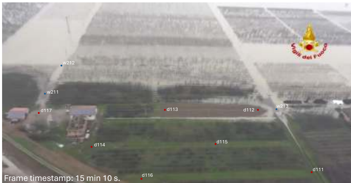
Figure S79. Frame of the aerial videography taken by the “Vigili del Fuoco” Fire Department of Modena. Wet points are highlighted in blue and dry points are highlighted in red. The time reported in the frame is counted from the beginning of the aerial videography occurred on 20 January 2014 at about 11:30 AM.
