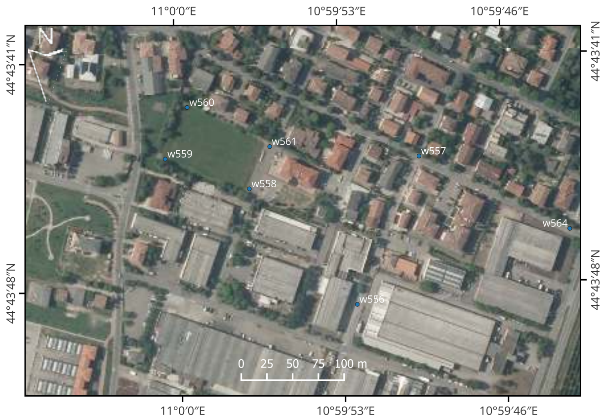
Figure S32. Orthoimage associated to the previous aerial videography frame, where georeferenced wet points are highlighted in blue and georeferenced dry points are highlighted in red.
