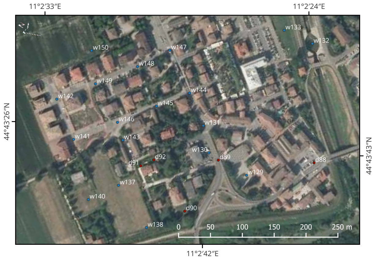
Figure S56. Orthoimage associated to the previous aerial videography frame, where georeferenced wet points are highlighted in blue and georeferenced dry points are highlighted in red.
