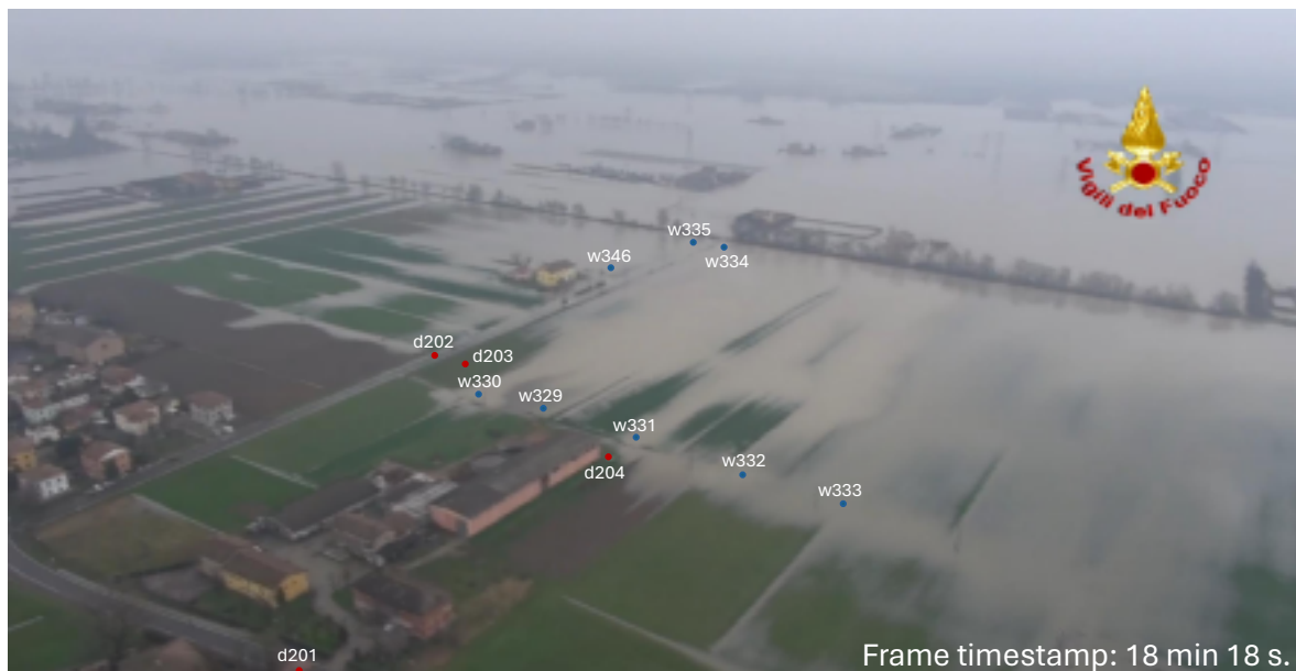
Figure S107. Frame of the aerial videography taken by the “Vigili del Fuoco” Fire Department of Modena. Wet points are highlighted in blue and dry points are highlighted in red. The time reported in the frame is counted from the beginning of the aerial videography occurred on 20 January 2014 at about 11:30 AM.
