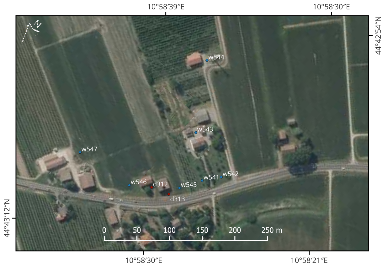
Figure S24. Orthoimage associated to the previous aerial videography frame, where georeferenced wet points are highlighted in blue and georeferenced dry points are highlighted in red.
