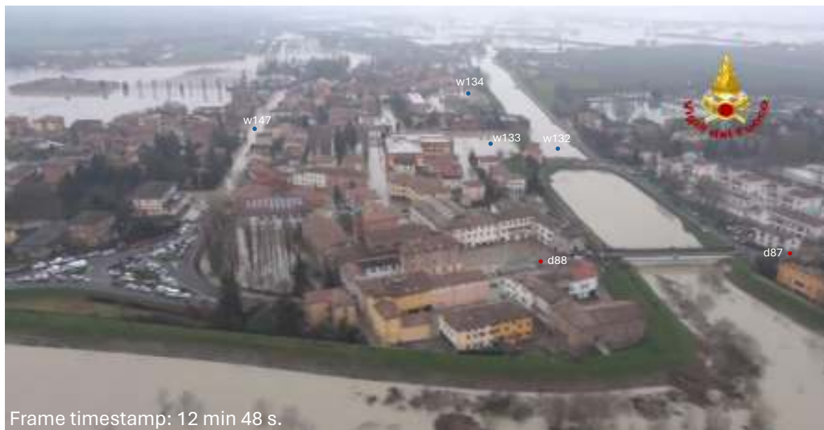
Figure S55. Frame of the aerial videography taken by the “Vigili del Fuoco” Fire Department of Modena. Wet points are highlighted in blue and dry points are highlighted in red. The time reported in the frame is counted from the beginning of the aerial videography occurred on 20 January 2014 at about 11:30 AM.
