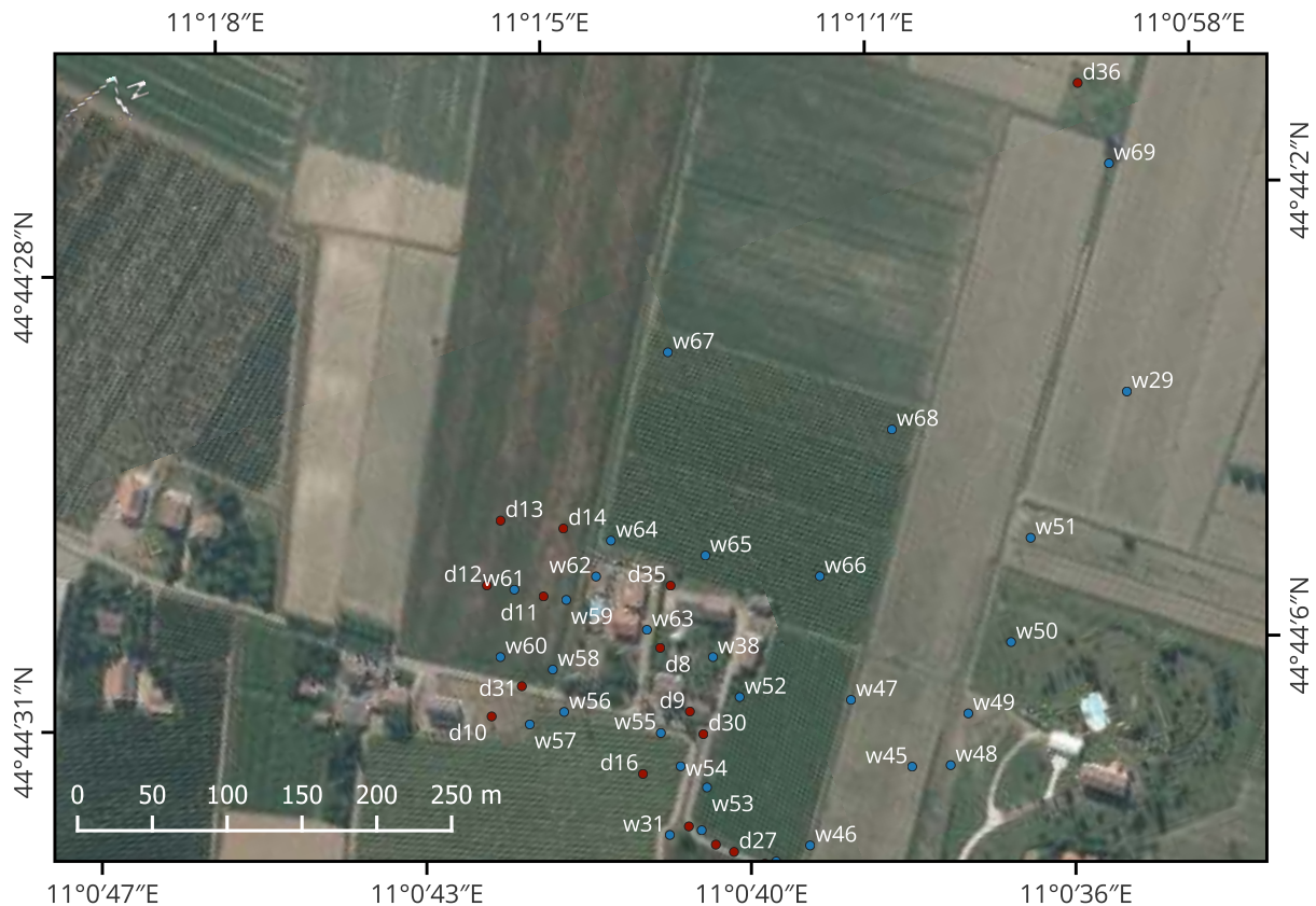
Figure S44. Orthoimage associated to the previous aerial videography frame, where georeferenced wet points are highlighted in blue and georeferenced dry points are highlighted in red.
