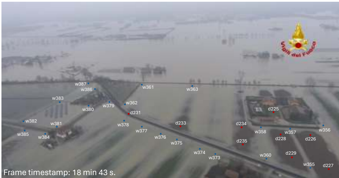
Figure S113. Frame of the aerial videography taken by the “Vigili del Fuoco” Fire Department of Modena. Wet points are highlighted in blue and dry points are highlighted in red. The time reported in the frame is counted from the beginning of the aerial videography occurred on 20 January 2014 at about 11:30 AM.
