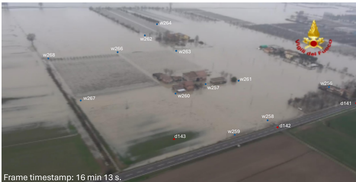
Figure S93. Frame of the aerial videography taken by the “Vigili del Fuoco” Fire Department of Modena. Wet points are highlighted in blue and dry points are highlighted in red. The time reported in the frame is counted from the beginning of the aerial videography occurred on 20 January 2014 at about 11:30 AM.
