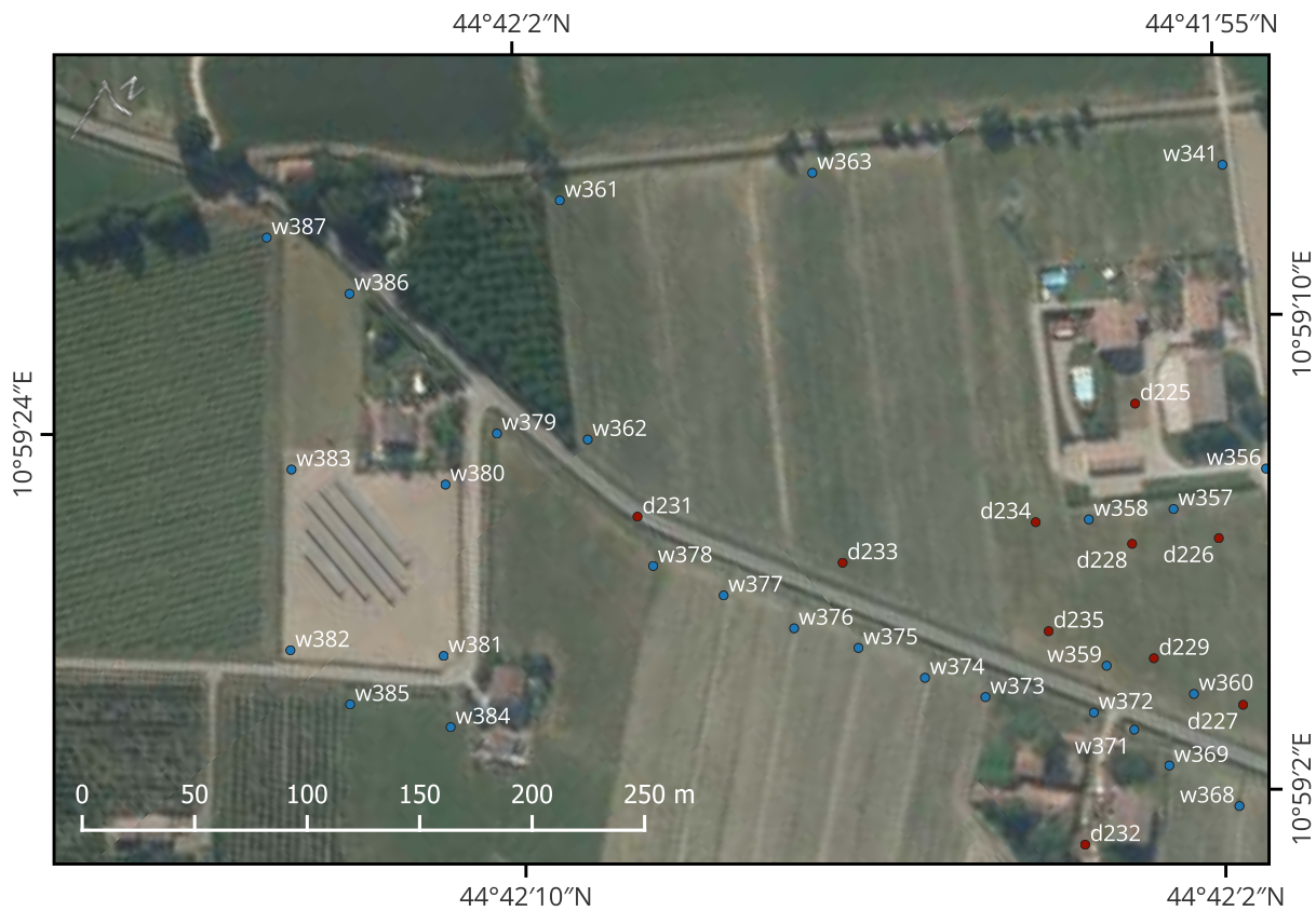
Figure S114. Orthoimage associated to the previous aerial videography frame, where georeferenced wet points are highlighted in blue and georeferenced dry points are highlighted in red.
