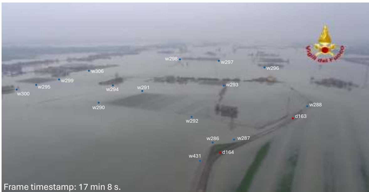
Figure S99. Frame of the aerial videography taken by the “Vigili del Fuoco” Fire Department of Modena. Wet points are highlighted in blue and dry points are highlighted in red. The time reported in the frame is counted from the beginning of the aerial videography occurred on 20 January 2014 at about 11:30 AM.
