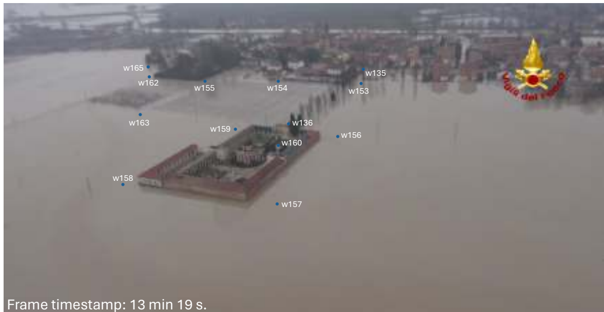
Figure S63. Frame of the aerial videography taken by the “Vigili del Fuoco” Fire Department of Modena. Wet points are highlighted in blue and dry points are highlighted in red. The time reported in the frame is counted from the beginning of the aerial videography occurred on 20 January 2014 at about 11:30 AM.
