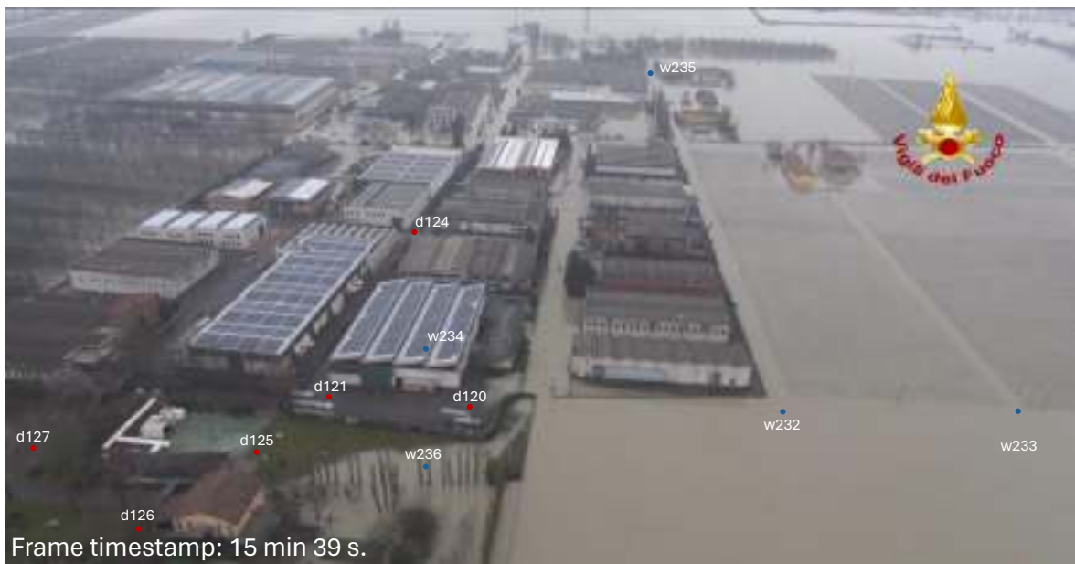
Figure S85. Frame of the aerial videography taken by the “Vigili del Fuoco” Fire Department of Modena. Wet points are highlighted in blue and dry points are highlighted in red. The time reported in the frame is counted from the beginning of the aerial videography occurred on 20 January 2014 at about 11:30 AM.
