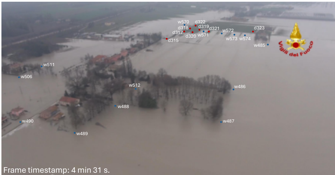
Figure S11. Frame of the aerial videography taken by the “Vigili del Fuoco” Fire Department of Modena. Wet points are highlighted in blue and dry points are highlighted in red. The time reported in the frame is counted from the beginning of the aerial videography occurred on 20 January 2014 at about 11:30 AM.
