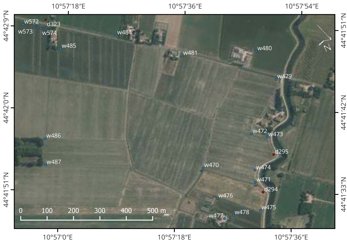
Figure S10. Orthoimage associated to the previous aerial videography frame, where georeferenced wet points are highlighted in blue and georeferenced dry points are highlighted in red.
