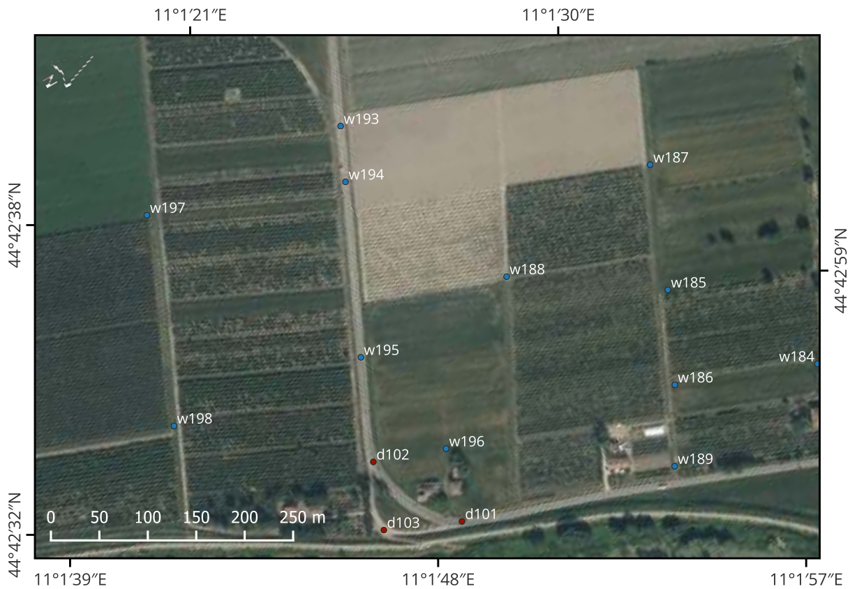
Figure S74. Orthoimage associated to the previous aerial videography frame, where georeferenced wet points are highlighted in blue and georeferenced dry points are highlighted in red.
