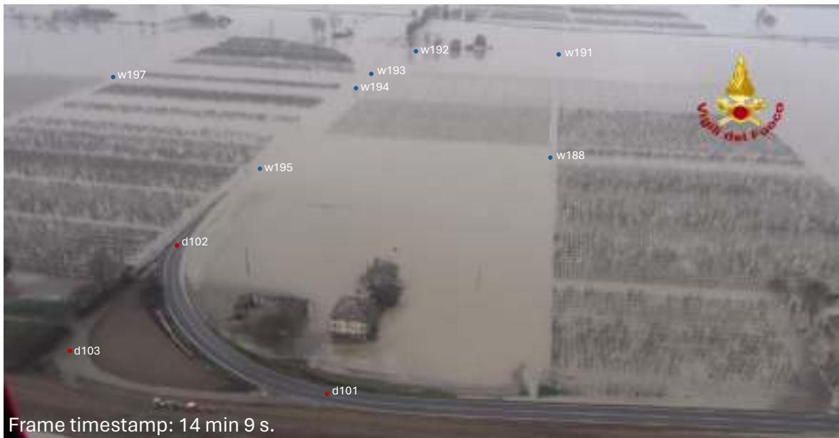
Figure S71. Frame of the aerial videography taken by the “Vigili del Fuoco” Fire Department of Modena. Wet points are highlighted in blue and dry points are highlighted in red. The time reported in the frame is counted from the beginning of the aerial videography occurred on 20 January 2014 at about 11:30 AM.
