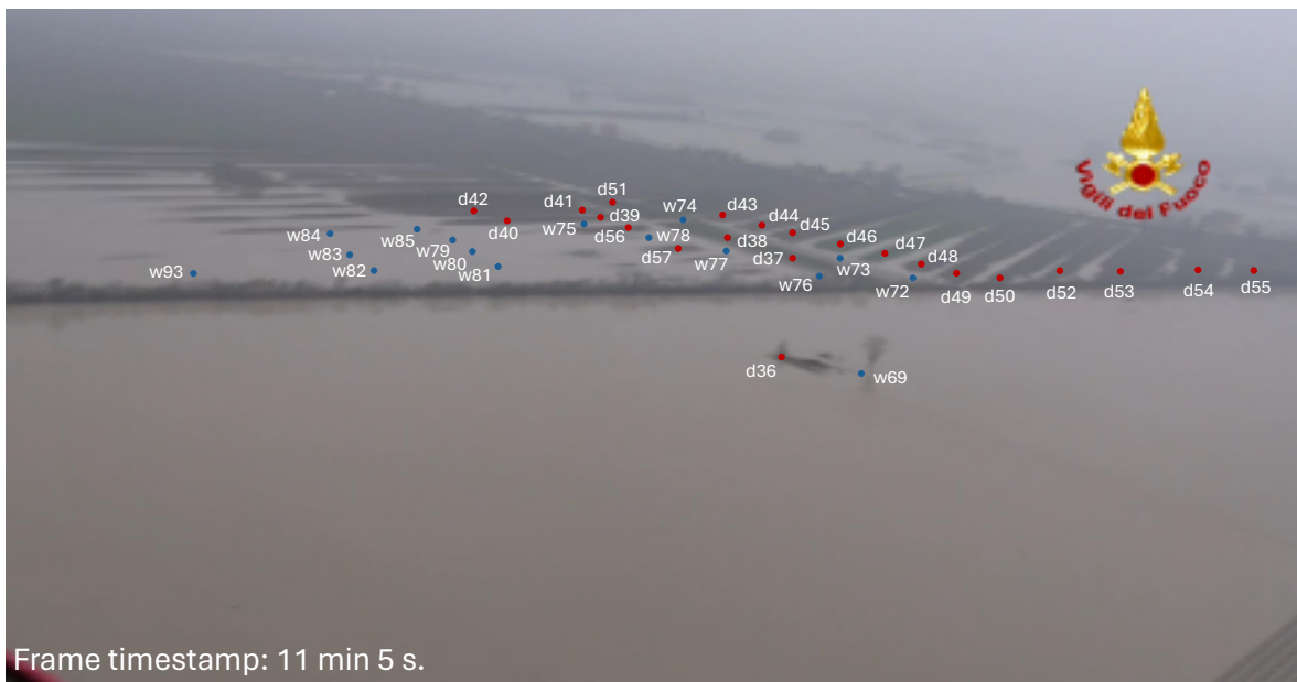
Figure S45. Frame of the aerial videography taken by the “Vigili del Fuoco” Fire Department of Modena. Wet points are highlighted in blue and dry points are highlighted in red. The time reported in the frame is counted from the beginning of the aerial videography occurred on 20 January 2014 at about 11:30 AM.
