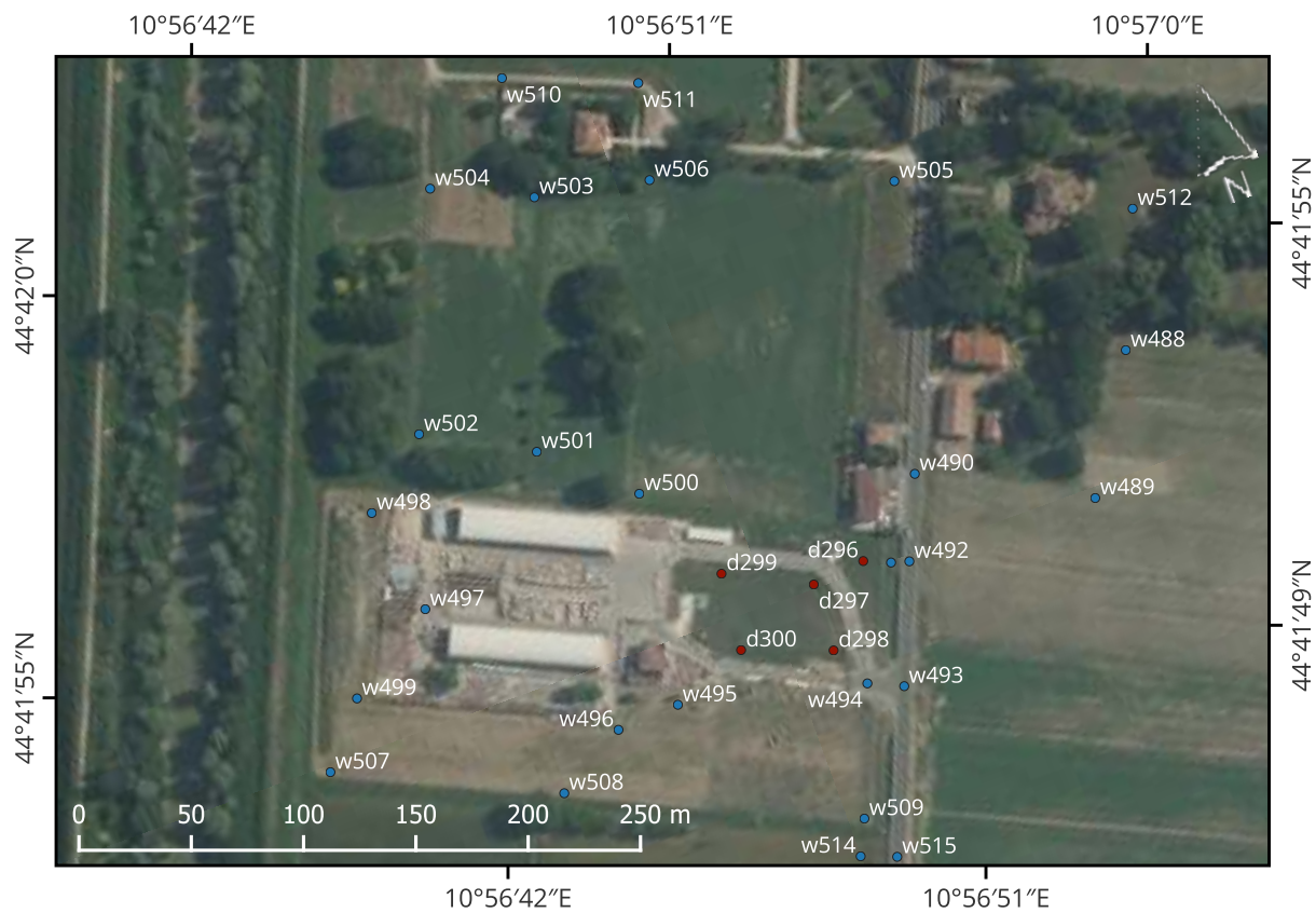
Figure S14. Orthoimage associated to the previous aerial videography frame, where georeferenced wet points are highlighted in blue and georeferenced dry points are highlighted in red.
