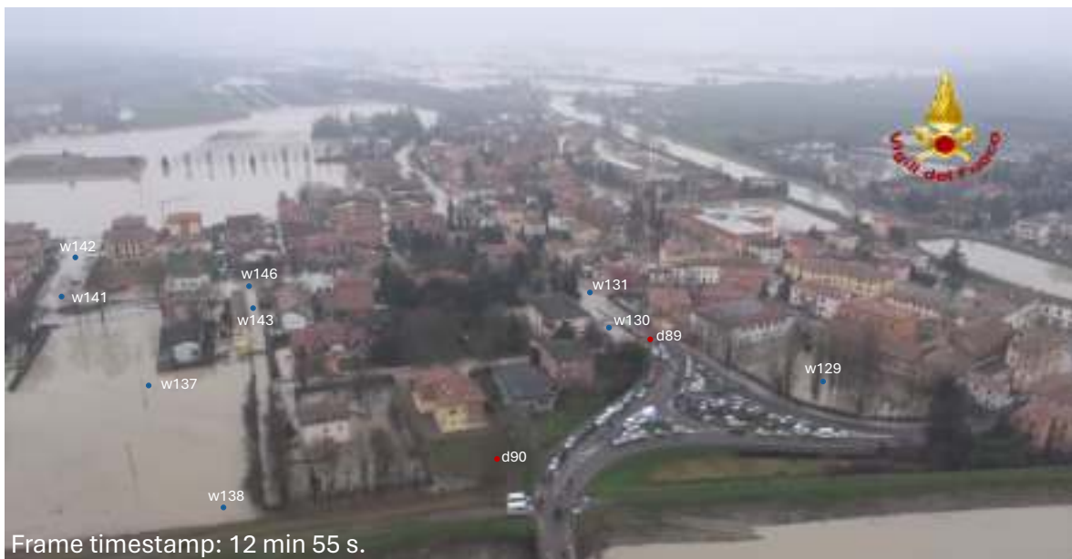
Figure S57. Frame of the aerial videography taken by the “Vigili del Fuoco” Fire Department of Modena. Wet points are highlighted in blue and dry points are highlighted in red. The time reported in the frame is counted from the beginning of the aerial videography occurred on 20 January 2014 at about 11:30 AM.
