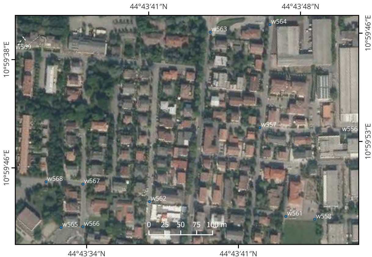
Figure S34. Orthoimage associated to the previous aerial videography frame, where georeferenced wet points are highlighted in blue and georeferenced dry points are highlighted in red.
