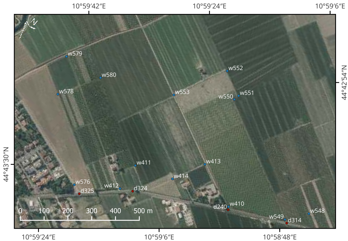
Figure S26. Orthoimage associated to the previous aerial videography frame, where georeferenced wet points are highlighted in blue and georeferenced dry points are highlighted in red.
