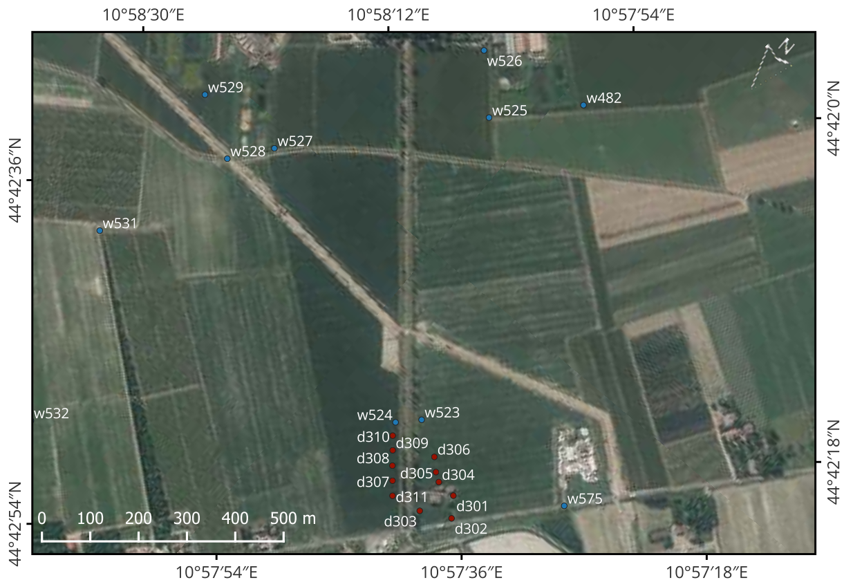
Figure S20. Orthoimage associated to the previous aerial videography frame, where georeferenced wet points are highlighted in blue and georeferenced dry points are highlighted in red.
