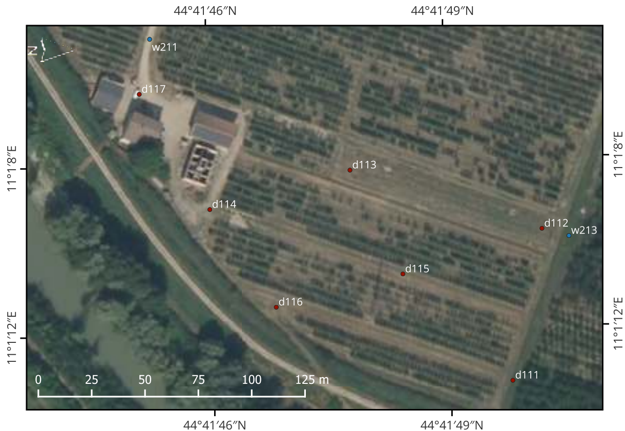
Figure S80. Orthoimage associated to the previous aerial videography frame, where georeferenced wet points are highlighted in blue and georeferenced dry points are highlighted in red.
