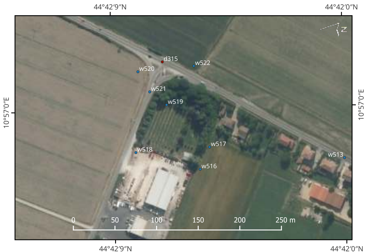
Figure S18. Orthoimage associated to the previous aerial videography frame, where georeferenced wet points are highlighted in blue and georeferenced dry points are highlighted in red.
