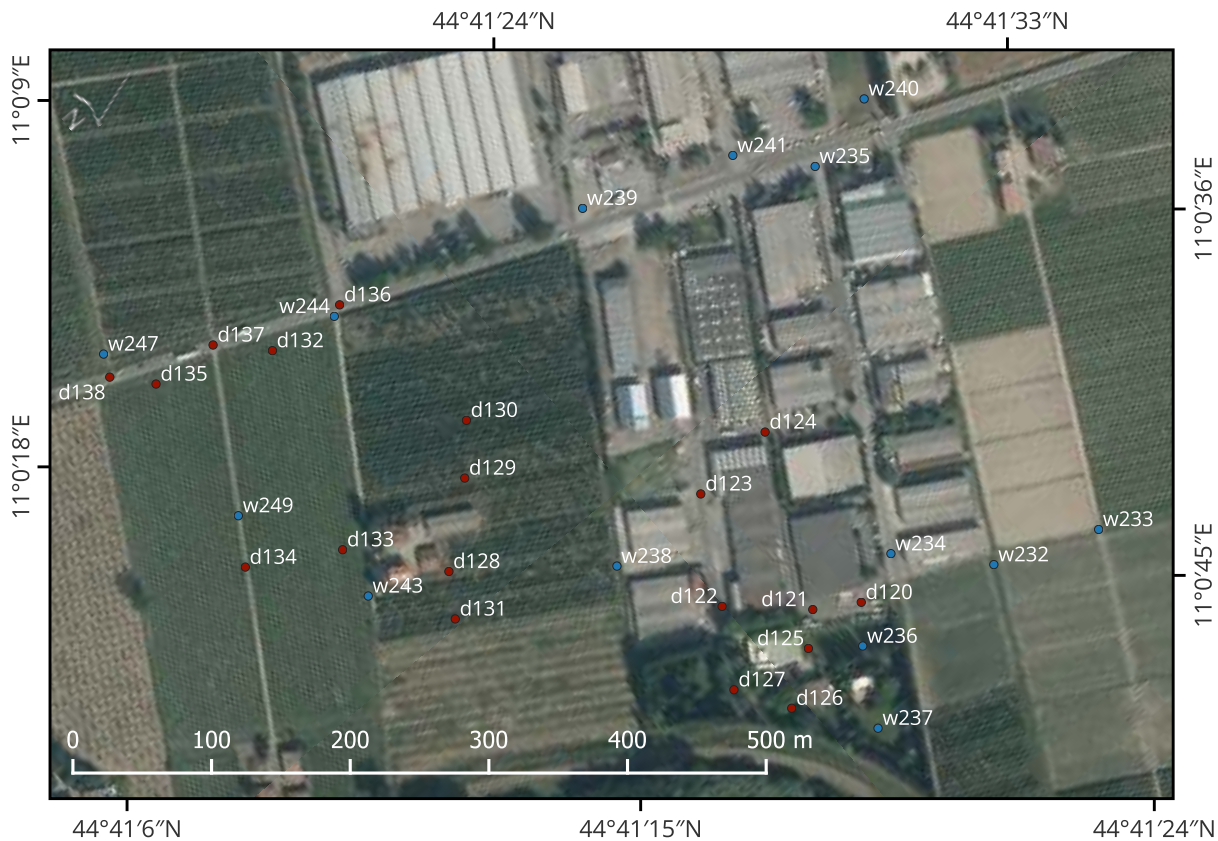
Figure S90. Orthoimage associated to the previous aerial videography frame, where georeferenced wet points are highlighted in blue and georeferenced dry points are highlighted in red.
