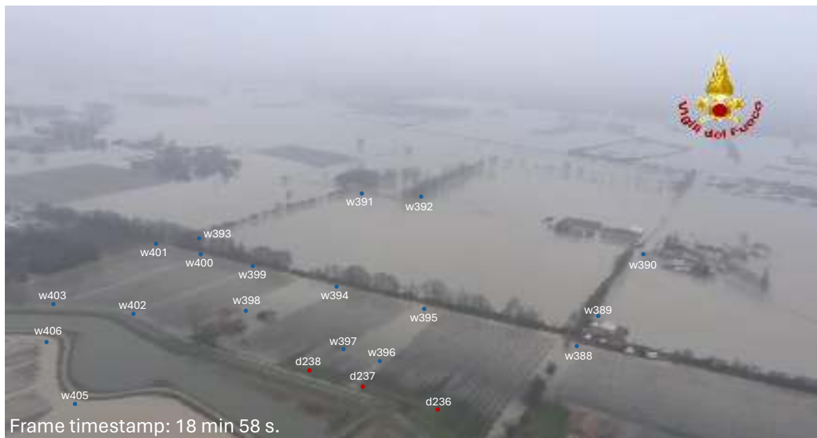
Figure S115. Frame of the aerial videography taken by the “Vigili del Fuoco” Fire Department of Modena. Wet points are highlighted in blue and dry points are highlighted in red. The time reported in the frame is counted from the beginning of the aerial videography occurred on 20 January 2014 at about 11:30 AM.
