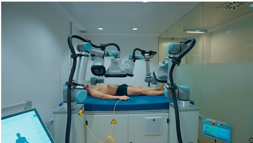
Figure 9. iToBoS prototype: European Horizon 2020 Intelligent Total Body Scanner platform integrating multiple high-resolution 2D cameras with liquid lenses, multispectral illumination, and AI-based data fusion to reconstruct 3D anatomical models for melanoma risk assessment.
