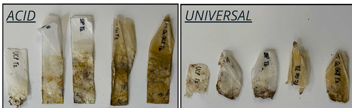
Fig. 9. Qualitative comparison between the samples after 28 days of burial in the two soil types.
