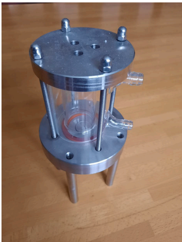
Fig. 1. measurement device for temperature dependent permittivity of liquids. From the top: cover with holes for insertion of temperature sensor and O-ring (not visible), heating/cooling jacket with inlet and outlet ports, truncated coaxial probe (from Agilent Dielectric Probe kit), O-ring and holding base.
