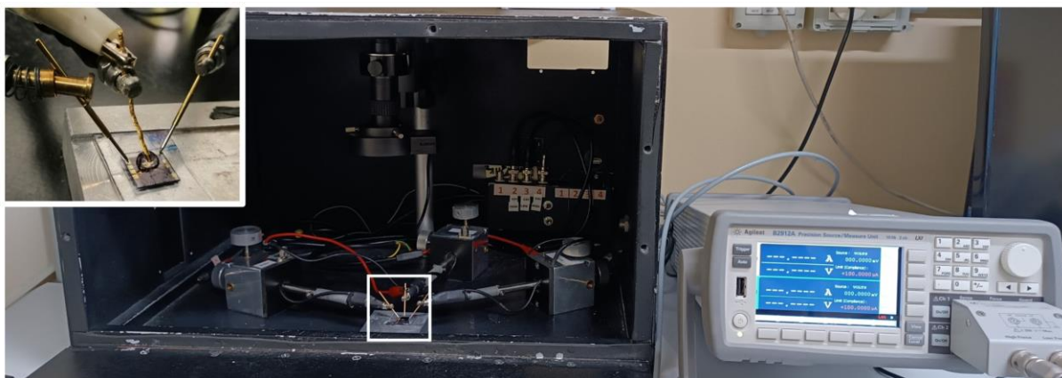
Figure 2.12. Electrical measurement instrument SMU (right) and Faraday cage (left). In the inset a zoom of the device with its electrical connections.
