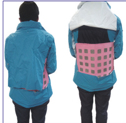
FIGURE 2: Real large textile antenna array deployed at user jacket backside.
