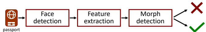
Fig. 2. A typical pipeline for S-MAD systems. The input is represented by the mugshot picture of the subject typically contained in the document, and the S-MAD algorithm outputs whether the given image has undergone a morphing process. Essentially, S-MAD methods consist of detectors of the artifacts produced by the morphing procedure.
