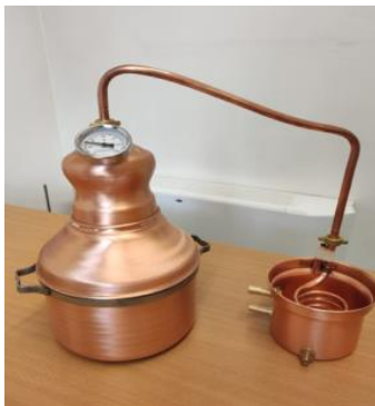
Figure 16: distiller still used for the extraction of essential oils.
