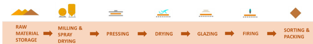
Figure 1 - Flow chart of the ceramic tile manufacturing process, elaborated upon from [230]
