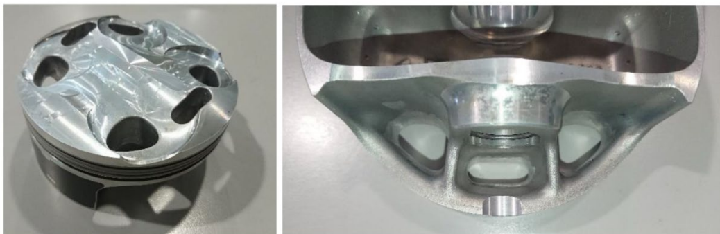
Figure 35 Pictures of the piston with holes.
