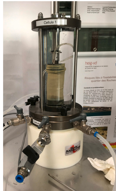
Fig. 4. Standard consolidated triaxial compression test performed on excavated soil specimen according to [35].
