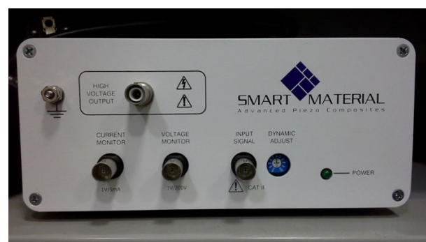
Figure 7. Voltage amplifier used after the MCU.
