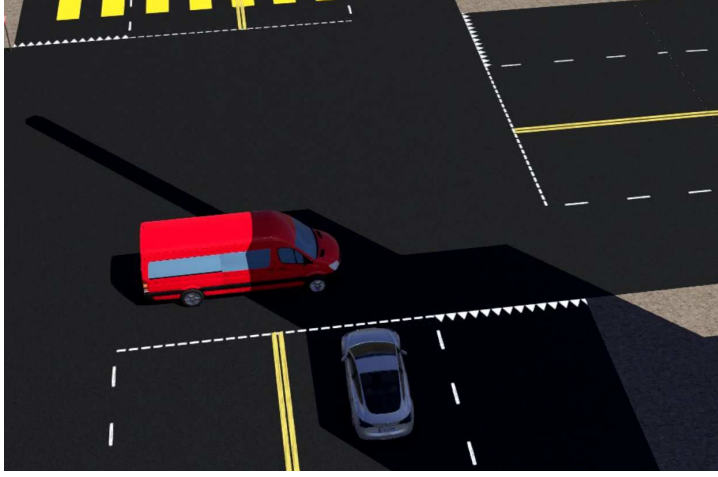
Figure 4.5: Webots simulation: the autonomous vehicle stops before entering an occupied intersection.
