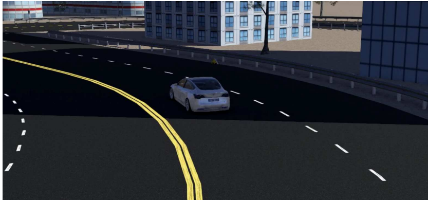
Figure 3.5: Lane-keeping scenario. The vehicle maintains a safe and adaptive distance from the road boundaries through the CBF-based lateral constraint. The safety margin is regulated by the parameter \lambda_L , ensuring smooth trajectory evolution without oscillatory behavior.
