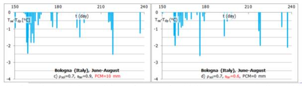
Figure 6. Risk of condensation for a) a typical cool roof, b) a cool roof coupled with 5 mm PCM, c) a cool roof coupled with 10 mm PCM, d) a cool roof with thermal emittance lower than usual.
