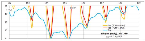
Figure 5. Time evolution patterns of dew point surface (with and without PCM) temperatures: the risk of condensation exists where the surface temperature falls below the dew point temperature.
