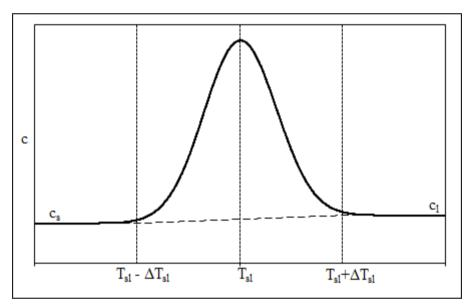
Figure 4. Effective specific heat of the PCM.
