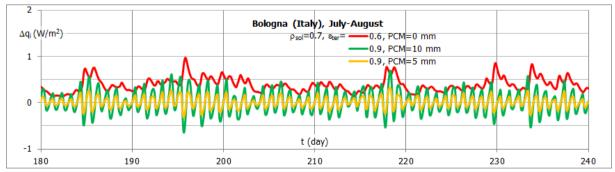
Figure 7. Change of the heat flowentering the inhabited space with respect to a typical cool roof with  $r_{sol}$  =0.7,  $e_{ter}$  =0.9.
