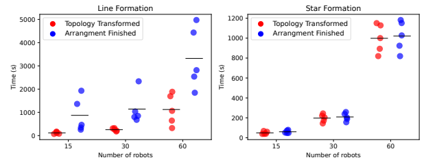
Fig. 3: Plots for the time taken to complete the tree transformation and arrangement completion, from randomly initial trees to the line and star formation, for 15, 30, and 60 robots.
