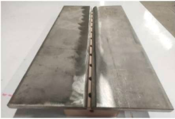
Fig. 6. Geopolymer weld backing in use, positioned beneath two stainless steel plates prepared for welding.
