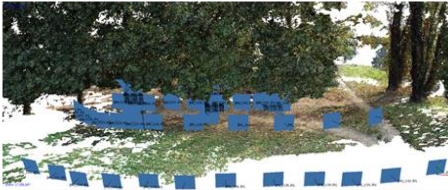
Figure 3. Dense point clouds of one of the investigated plots (APS model view), the blue squares represent the locations from which each of the images was taken.
