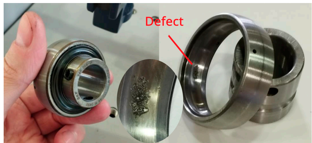
Figure 3. Detailed view of the damaged bearing: (left) assembled SKF YAR 204 2F unit; (right) disassembled outer race highlighting the localized defect (approx. 5 \times 3 mm); (center) magnified detail of the spalling area.
