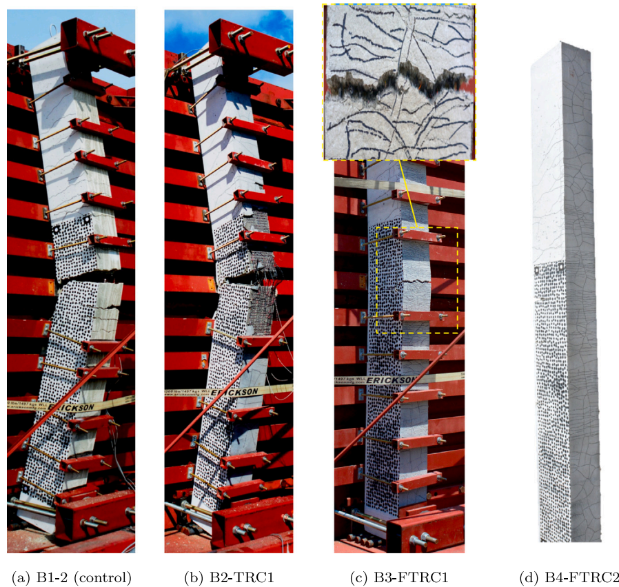
Fig. 8. Photographs depicting the progression of damage in beams after Blast 4.
