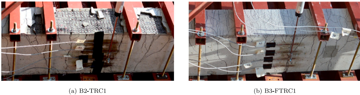
Fig. 7. Appearance of the mid-span after Blast 3 showing the influence of the addition of short fibers regarding the crack pattern and spalling retention.
