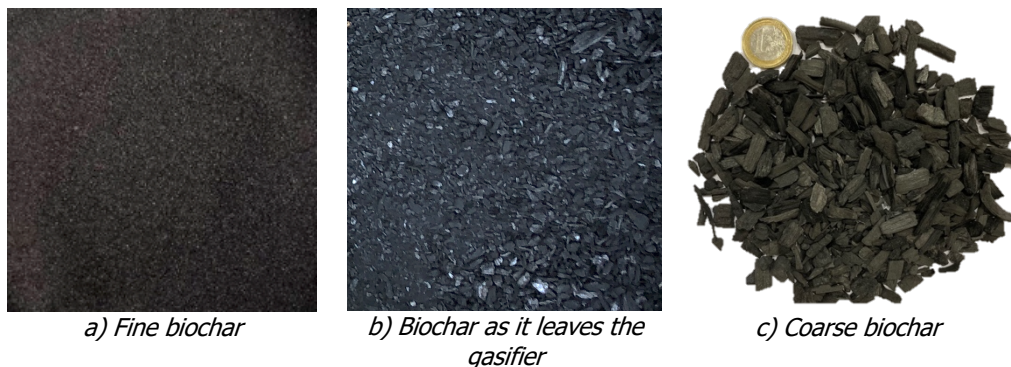
Figure 6-3. Some samples of biochar with different grains dimensions and different particle size distribution: from fine grains, a), to coarse grains, c).
