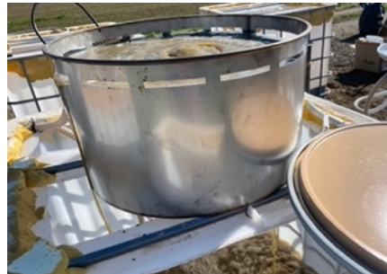
c) complete system on the left, reactor full of slurry on the right. The slots for the overflow discharge can be seen near the upper limit.
