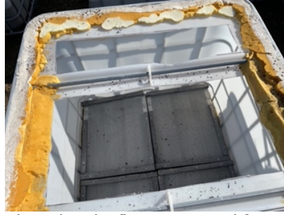
a) complete system on the left, mats in the tank on the right. The floating external frame and the plastic net that allows biochar-slurry contact are clearly recognizable
