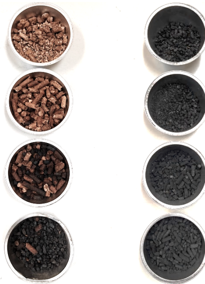
Figure 5-5. Biomass and biochar samples taken at different heights on the vertical of an All Power Labs Inc downdraft gasifier located in laboratory [64]. The conversion stages, from virgin biomass (in this case A1 pellets) to biochar, firstly through pyrolysis and after through gasification, are clearly visible. (The four samples on the left continues with the four samples on the right).
