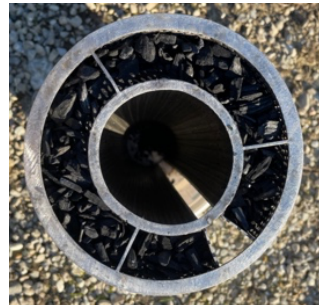
b) complete system on the left, detail of the filter filled with biochar on the right. The cut on the side has been created to facilitate the passage of the slurry into the filter.
