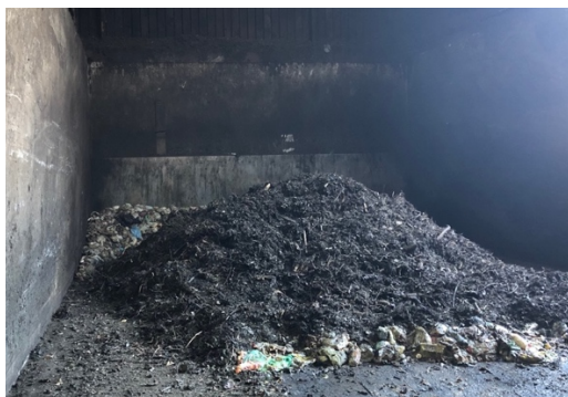
Figure 13-3. OFMSW and "bulk-wood" before mixing in the composting facility.
