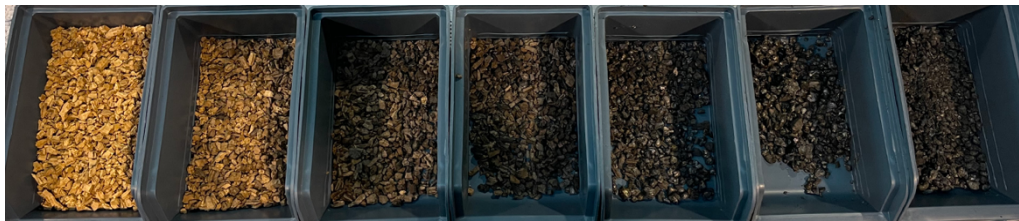
Figure 5-7. Evolution of cork subjected to pyrolysis in the absence of oxygen, processed through a small vessel laboratory pyrolizer. The progress of biomass conversion, from the left to the right, can be observed.
