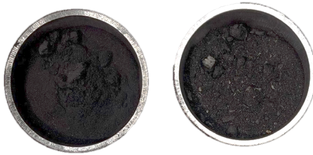
Figure 1-4. a) the apparatus used for measuring the EC under compression; b) two of the samples tested: on the right the biochar as-it-is after the gasification process, on the left the same biochar after grinding treatment.
