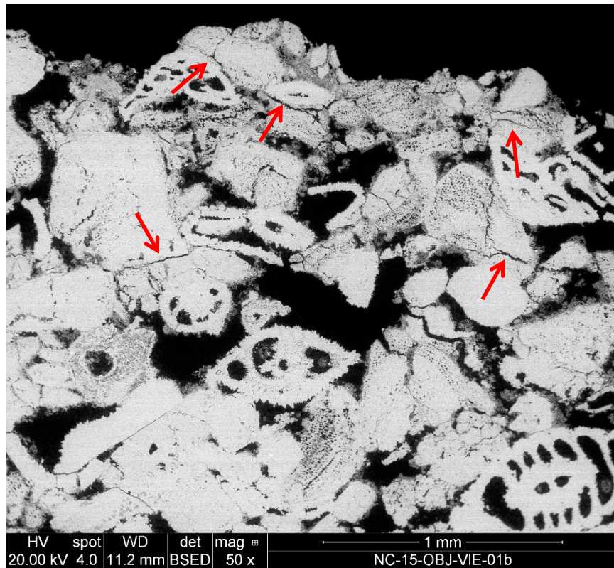
Figure S4. SEM-BSE, overview of the surface and subsurface zone exhibiting cracks parallel to the surface and between the fragments.
