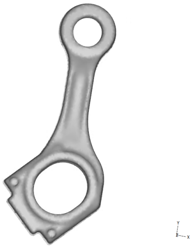
Near net-shape after profile machined by CNC
