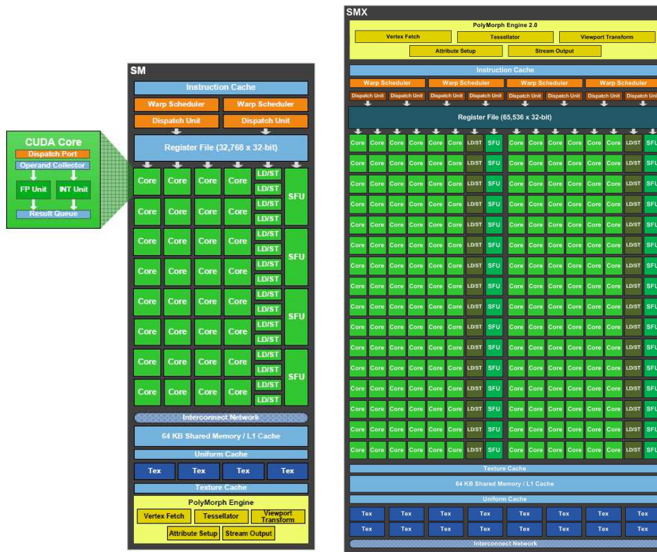
Figure 3.1: Theoretical scheme of a Streaming Multiprocessor (SM) on the left and of a Streaming Multiprocessor eXtreme (SMX) on the right.
