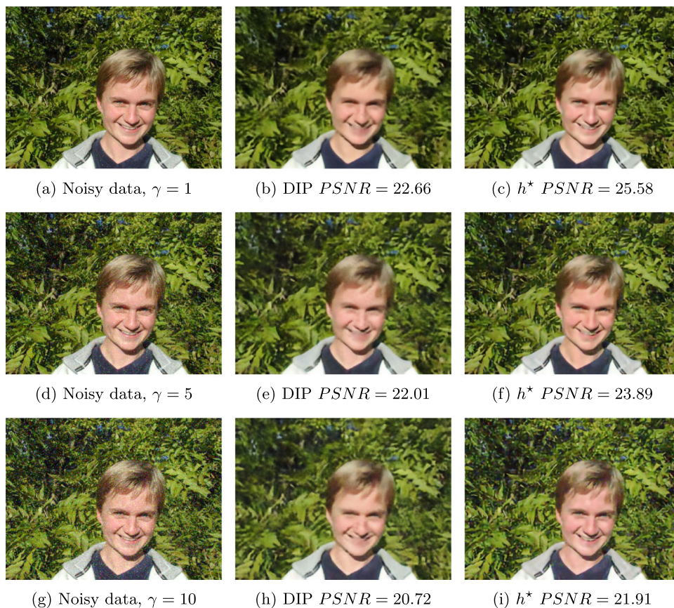
Fig. 8 Results achieved on Fig. 6b corrupted by Cauchy noise for \gamma = 1 (top row), \gamma = 5 (middle row) and \gamma = 10 (bottom row) via standard DIP (second column) and DIP with the best configuration reported in Table 8 (third column)
