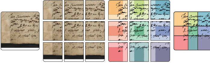
Figure 3.2: We combine the predictions of our model on overlapping patches at each point based on the distance between the point of interest and the center of each patch so that the artifacts at the patches borders are reduced.
