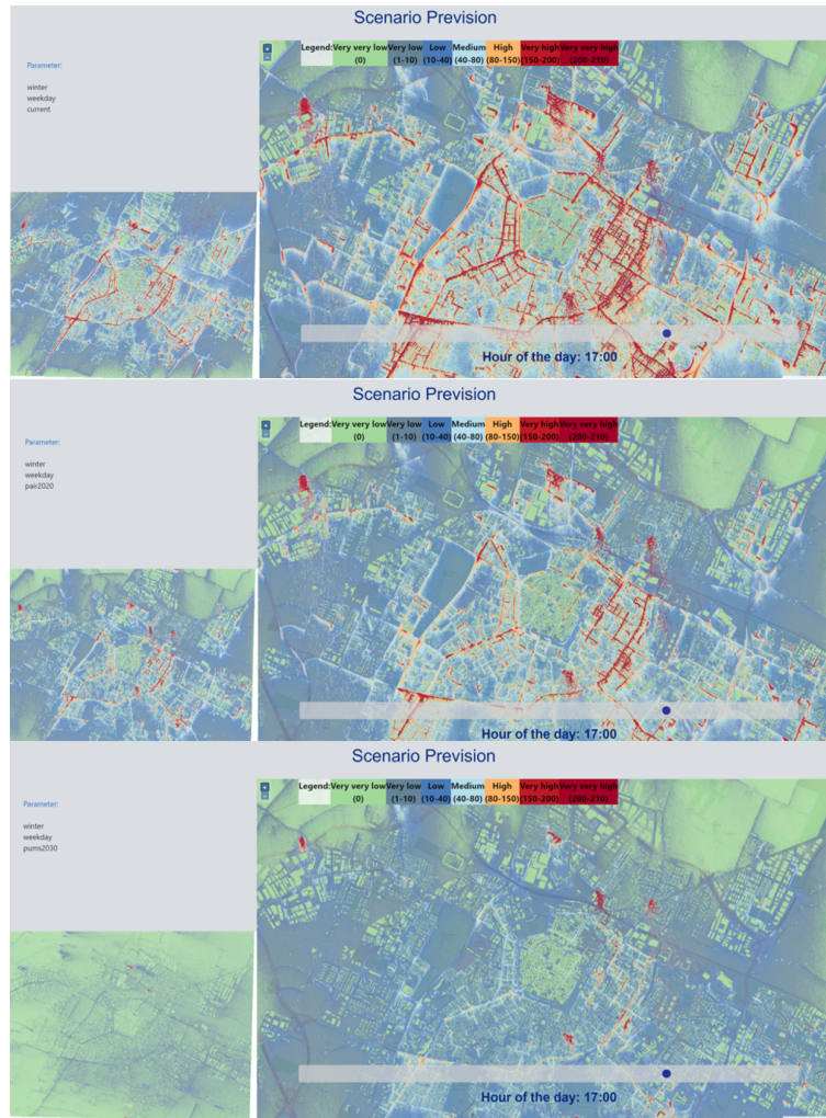
Fig. 14 Comparison of winter weekdays in 3 different scenarios: with current vehicles fleet (top), with Pair2020 vehicles fleet (middle), and with PUMS 2030 vehicles fleet (bottom). The image refers to the city of Modena
