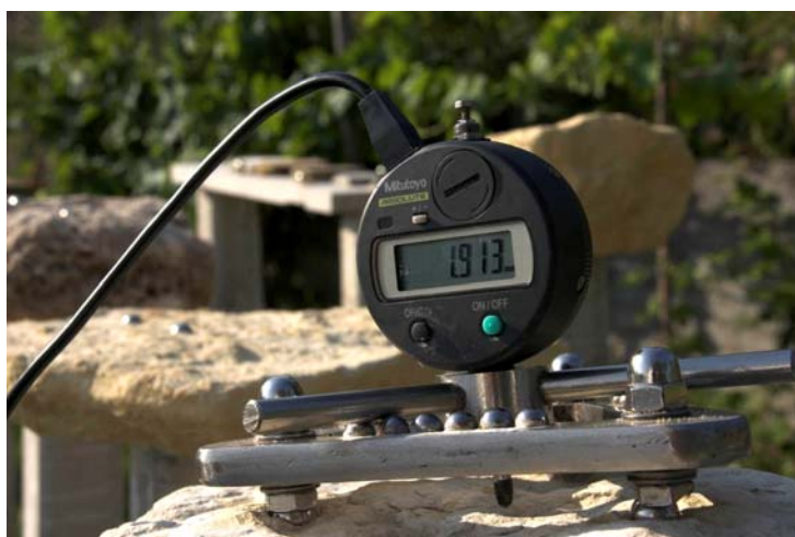
Fig. 1: The TMEM on the samples of the experimental station in Muggia, Trieste (I).
