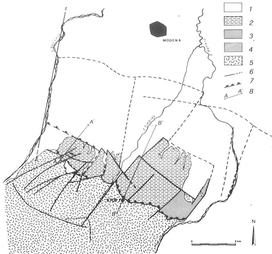
Fig. 1 - Geological sketch map of the margin of the Apennines between the rivers Panaro and Secchia. 1) Alluvium; 2) Marine-continental Pleistocene formations; 3) Upper Pliocene formation; 4) Early Pliocene formation; 5) Pre-Pliocene formations; 6) Faults; 7) Flexure; 8) Geological cross-sections line.
