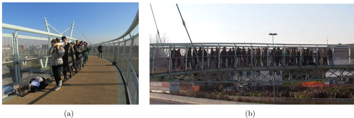
Figure 3.6: Examples of dynamic tests: (a) 12 pedestrians walking in single file on the north side of the deck and (b) 44 pedestrians walking in a closed loop on the main span
