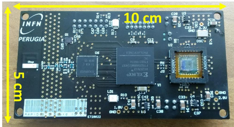
Figure IV-26: The implementation of the final Prototype 2: the chip antenna is placed in the left region, the CPLD and SoC are in the middle and the CMOS image sensor is on the right of the picture
