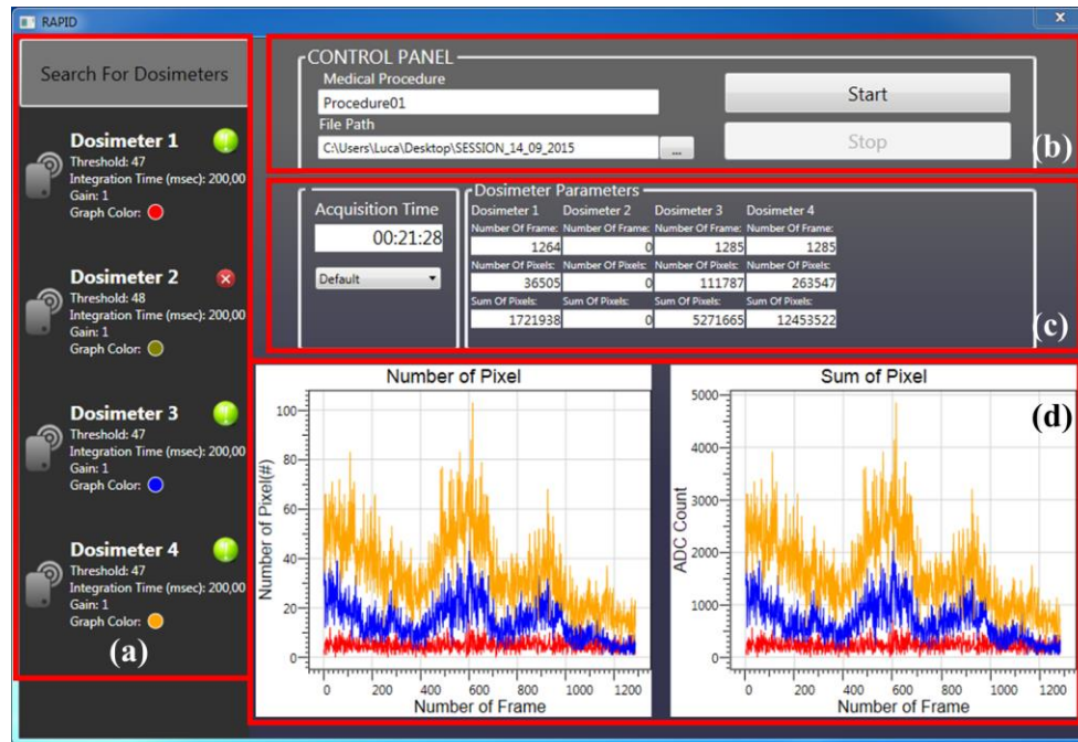
Figure IV-9: Screenshot of the main control window of the GUI implemented in the remote terminal: (a) the list of the available dosimeters are displayed with the status of configuration; (b) the buttons “Start and Stop acquisition” that control the data acquisition procedure; the text box is used for defining the kind of IRad procedure; (c) the information of the acquisition status of all the configured dosimeters; (d) the real-time graphical monitoring.
