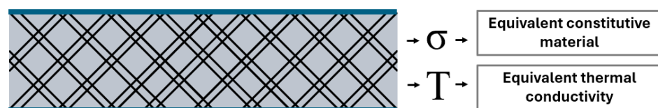
Figure 4. Sandwich panel model representing the outer layer of multifunctional lattice for mesoscale design.
