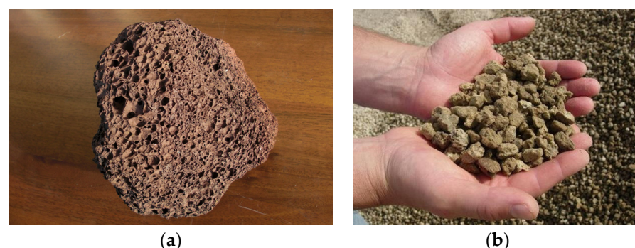
Figure 2. Lapillus (a) and zeolitic tuff (b) [16].
