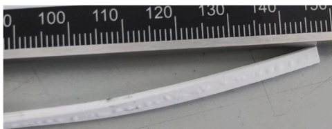
Fig. 9. Blisters on the surface of the feedstock 4 sample after 3 hours water debinding at 40°C.
