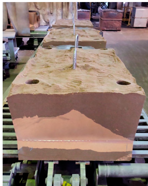
Figure 9. Sample mould in normal production with the layers close to the parting surface, the cavity inside formed with virgin sand, and the rest filled with reused sand.
