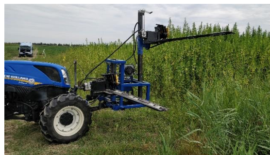
Figure 2: Prototype for the hemp harvesting, front bars with in evidence the blades for the two cutting heights
