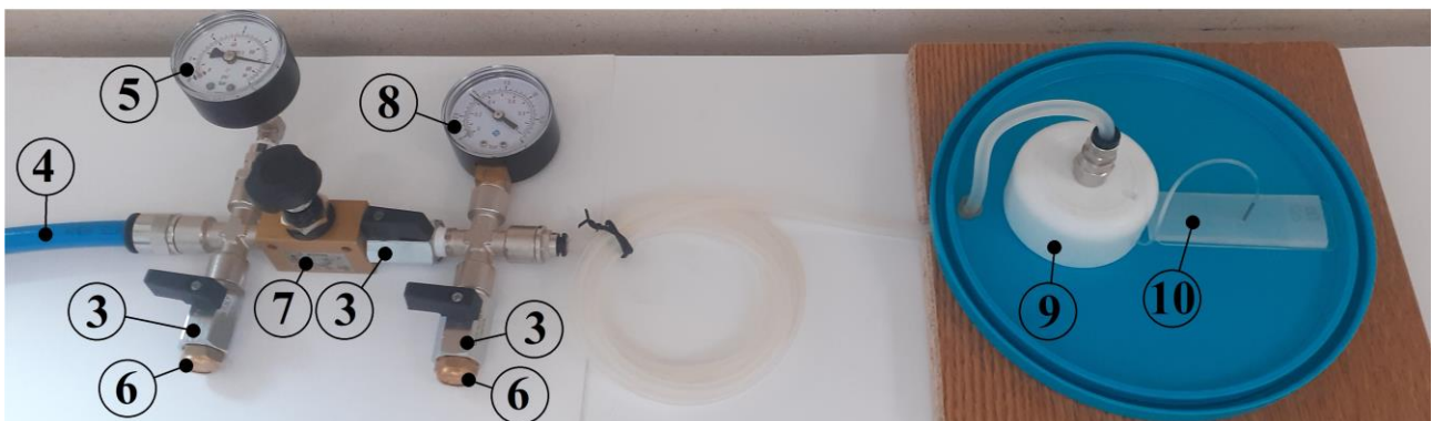
Fig. 5.2.9. Pressure generator. (1) Air inlet from the manual pump. (2) One-way valve. (3) Manual valve. (4) Air hose as high-pressure air reservoir. (5) 0-6 bar manometer. (6) Vent. (7) Air restrictor. (8) 0-1 bar manometer. (9) Air-water reservoir. (10) Test device.
