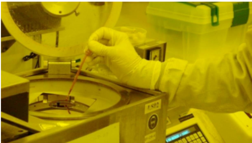
Fig. 3.2.1. Manual application of photoresist to a blank mask before using the spin coater inside a cleanroom with yellow lighting [49].
