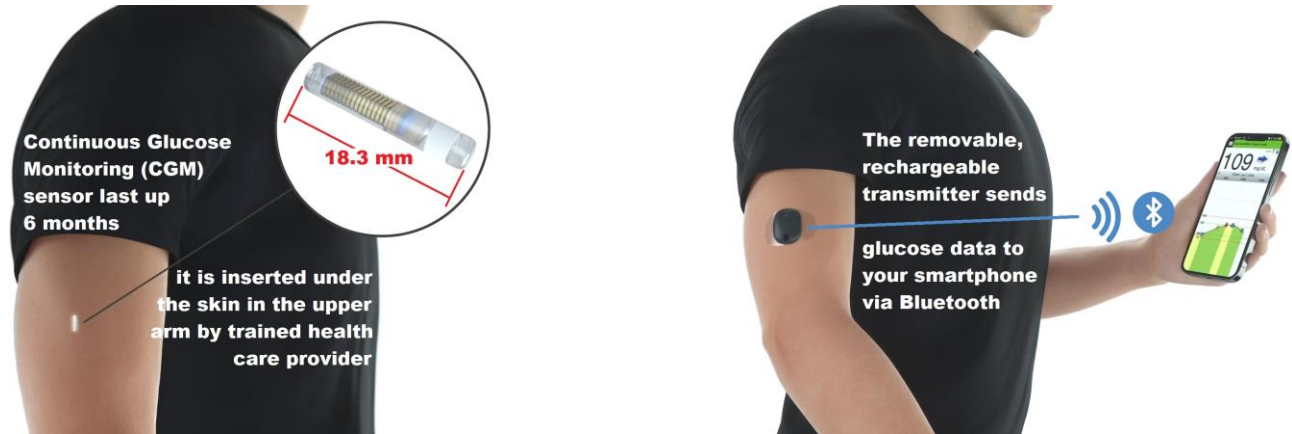
Fig. 1.3.6. A wearable Continuous Glucose Monitoring (CGM) system (redraw from [18]).
