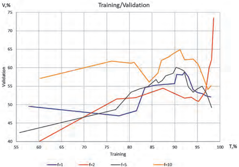
Fig. 2. Measurement accuracy dependences during ANN training of validation database (V, %) on the discrimination accuracy of training database (T, %) for different sampling rates ( f = 1, 2, 5, 10 ) of FVT and various number of interframe difference accumulations f = 1 — FVT sampling frequency 1Hz, for 10 interframe difference accumulations; f = 2 — FVT sampling frequency 2Hz, for 25 interframe difference accumulations; f = 5 — FVT sampling frequency 5Hz, for 25 interframe difference accumulations; f = 10 — FVT sampling frequency 10Hz, for 25 interframe difference accumulations
