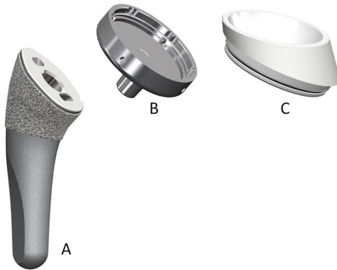
Figure 14. Short stem lateralized humeral component of reverse shoulder arthroplasty. A) a hydroxyapatite-coated curved short stem 132.5^\circ inclination; B) an eccentric (+ 1.5 mm and + 3.5 mm) reverse tray; and C) an asymmetric polyethylene insert (thickness + 6 mm and + 9 mm) with 12.5^\circ inclination.
