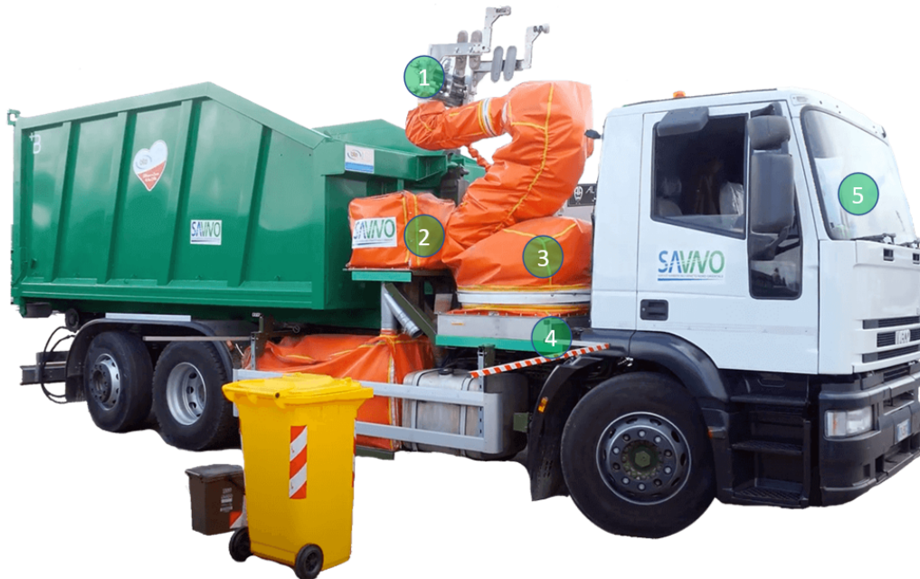
Figure 5.1: Overall structure of the Robish system for automated picking of urban waste.
