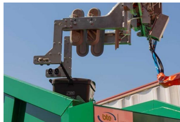
Figure 5.26: Handle release action
