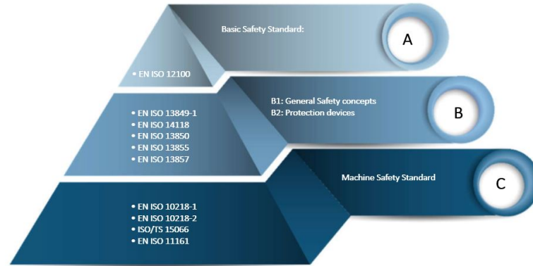
Figure 1.4: European Machinery Directive: the harmonised standards
