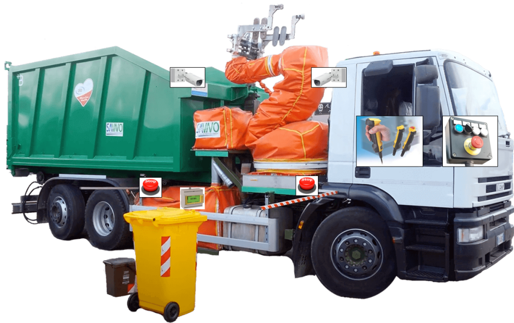
Figure 5.15: Robish system with external safety devices remarks
