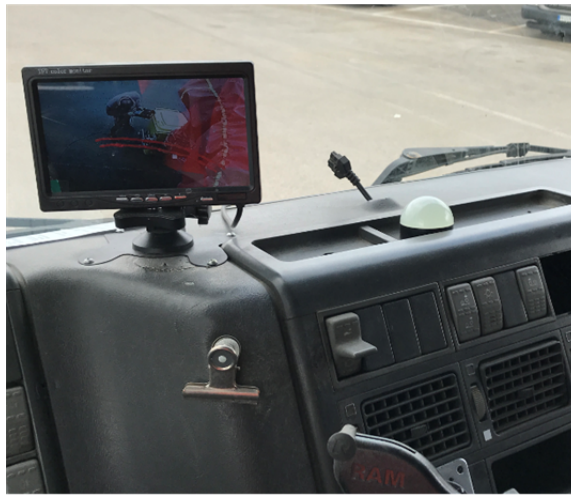
Figure 5.17: Closed circuit monitor of one cameras and the internal led light signaling
