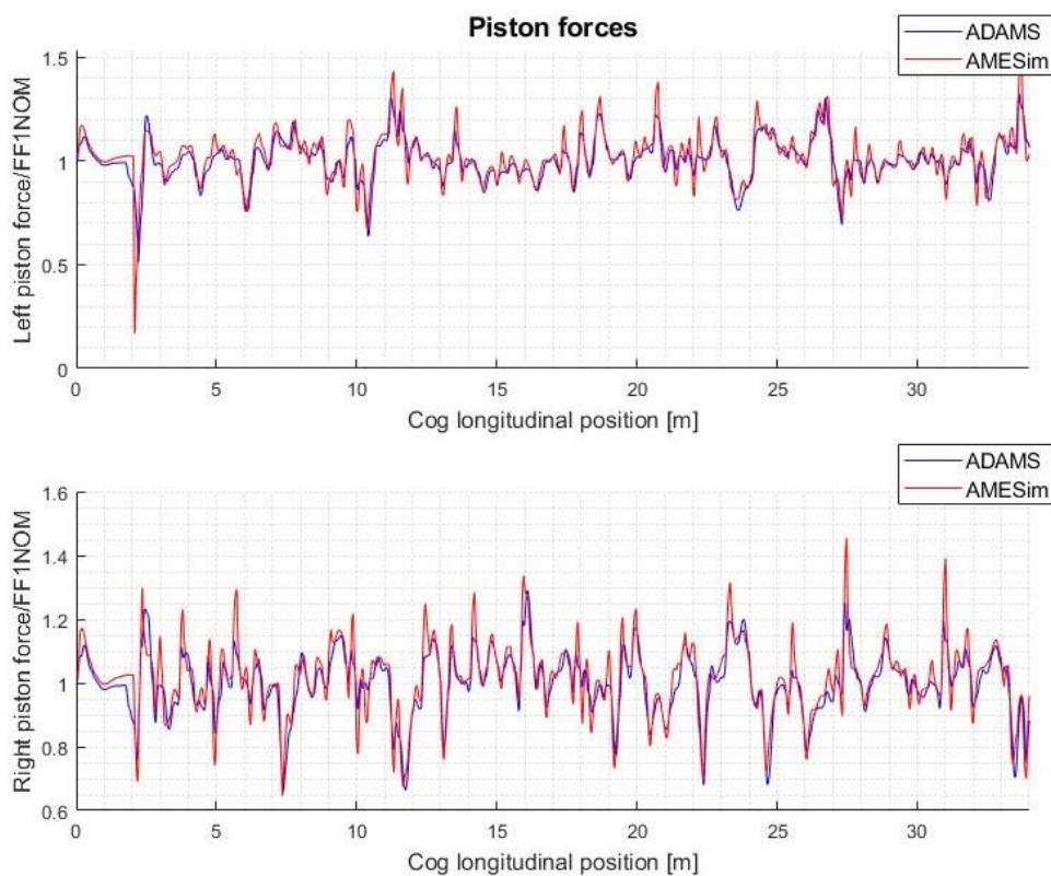
Figure 1.54: Dimensionless forces on suspension cylinders with the ISO 5008 test: Adams® (in blue) vs Amesim® (in red)
