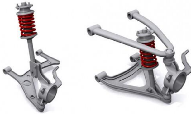
Figure 1.2: Two example of independent suspension architecture: MacPherson type (left) and double wishbone type (right)
