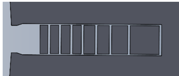
Fig. 1- Example of 8 asymmetric hairpins within a slot
