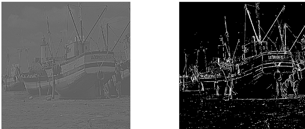
Figure 9: The image of the boat has been treated with one step of the algorithm (22) ( \gamma = -8 ) and a passage of the cut off procedure (28) with \tau = 165 .
