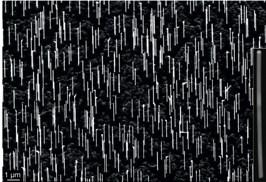
FIG. 2.1: SEM picture of nanowires as grown on a substrate. Insert shows a Scanning Transmission Electron Microscope image of a nanowire, with the gold seed nanoparticle visible on top.
