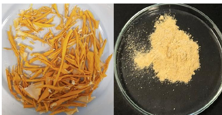
Figure 6 - Winter melon peel oven dried at 40 °C for 48 h, before (left) and after grinding (right).
