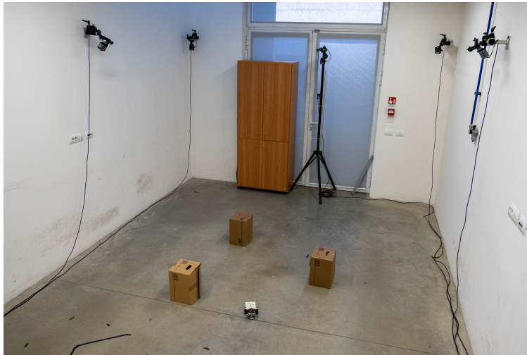
FIGURE 2.25: Testing environment composed of a motion capture system estimating the poses of the robot and the pushed object.
