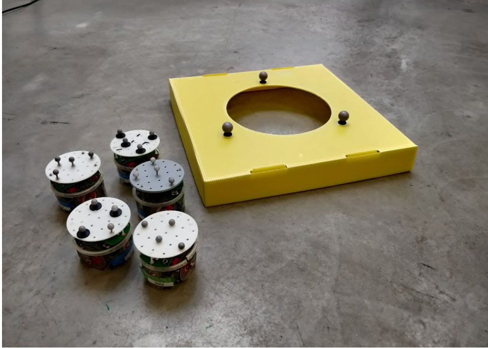
FIGURE 4.1: E-Puck robots approaching a square object to apply a pushing action inside the motion capture arena.
